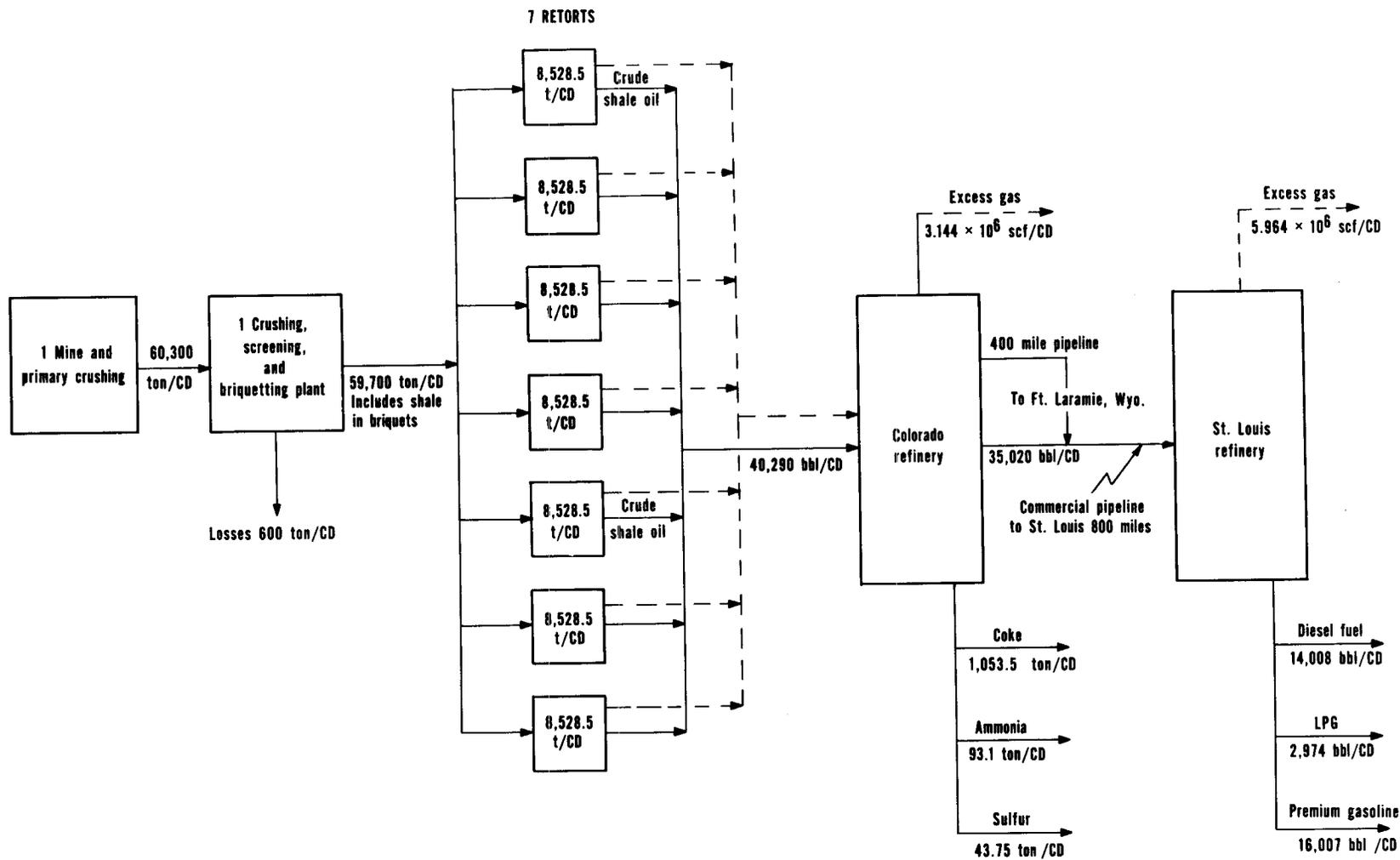
FIGURE 1. - General Block Diagram, Shale Oil Project (1966)
