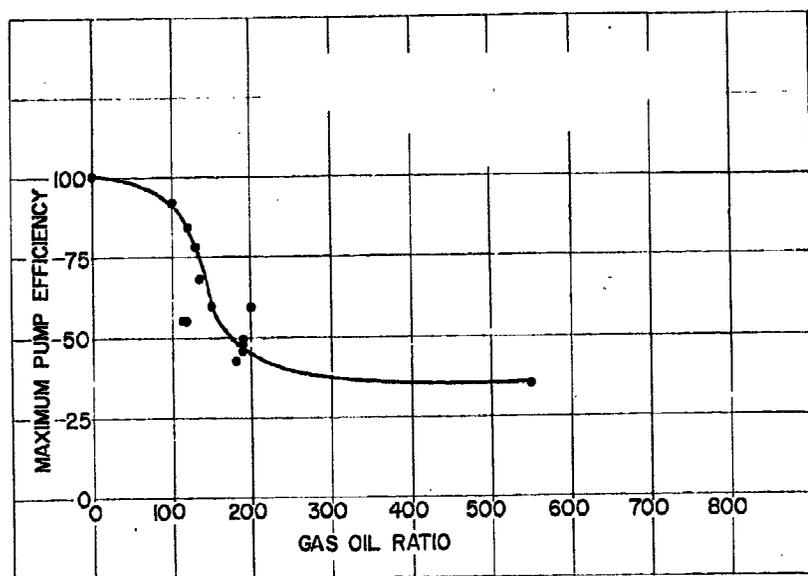
Fig. 1—Maximum possible pump efficiency, effect of GOR on well fluid gradient.
