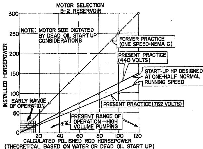
Fig. 2—Motor selection, B2 reservoir.
