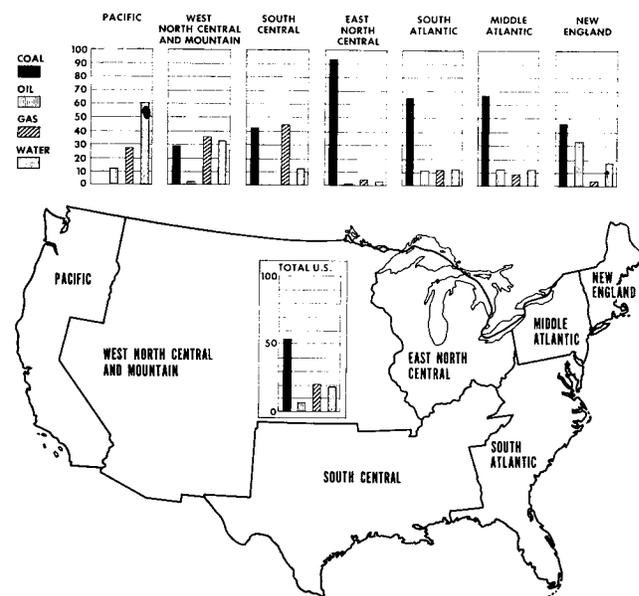
Fig. 4—Energy consumed in electric power generation, 1959.
