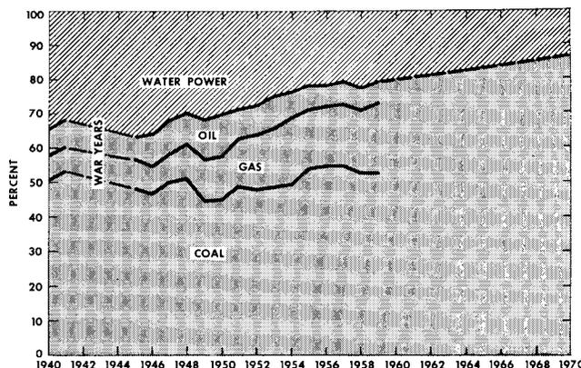
Fig. 3—Energy consumed for electric power generation (per cent of total each source).
