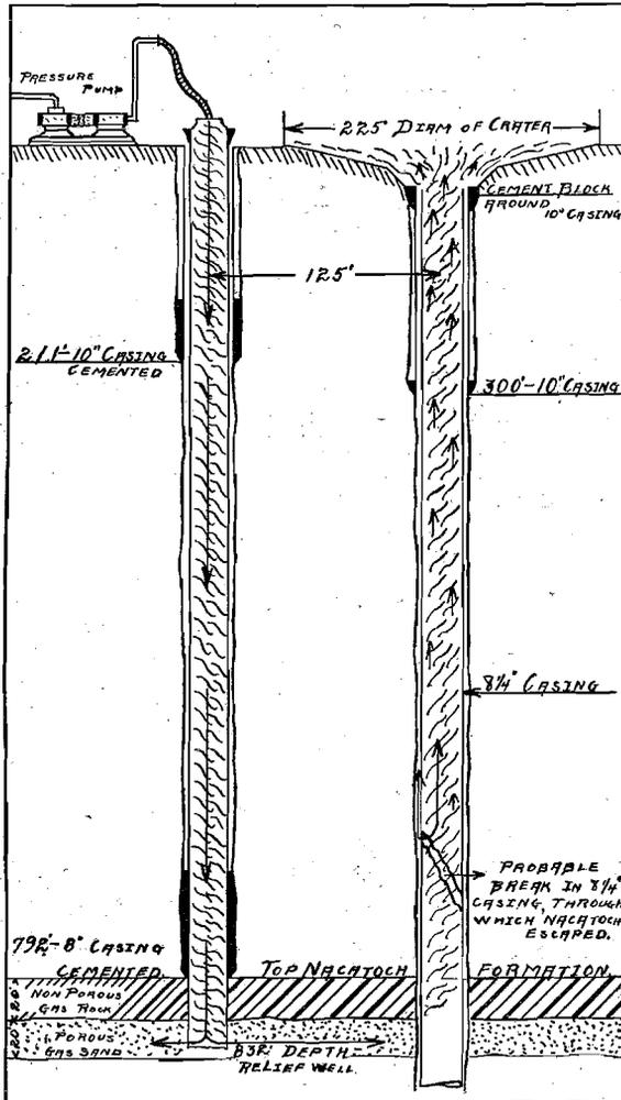
FIG. 5.—SECTION THROUGH BURNING WELL AND RELIEF WELL.
