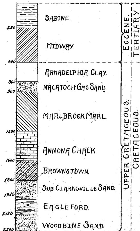
FIG. 2.—LOG AND SECTION OF A CADDO WELL.
