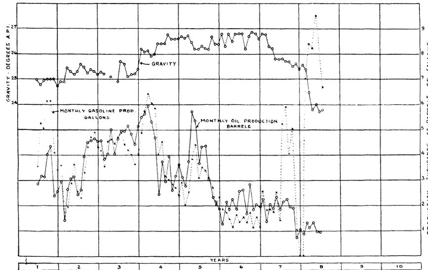
FIG. 5.—EFFECT OF A VACUUM ON THE CASINGHEAD.
