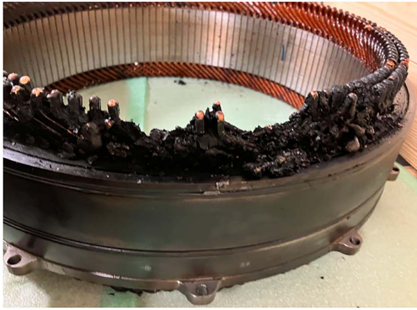
Fig. 2 Stator with severe damage
