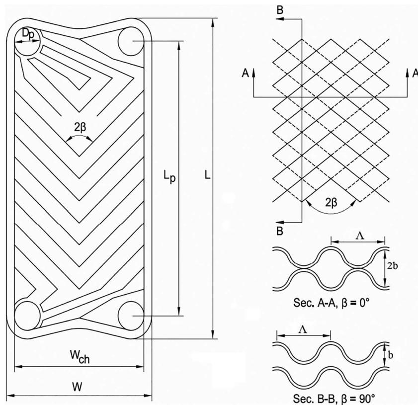
Fig. 1 Schematic of corrugated plate heat exchangers [3]
