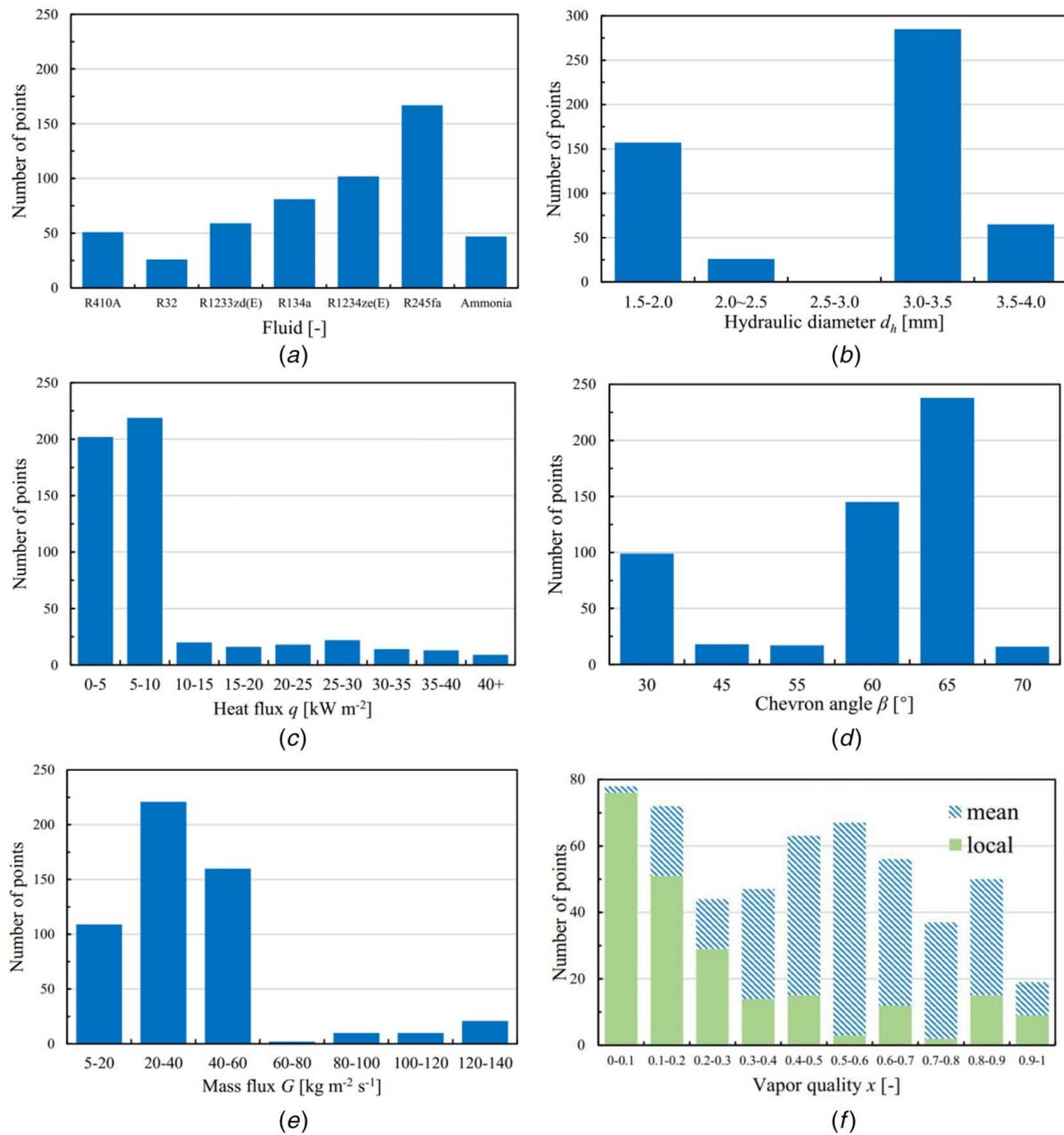
**Fig. 2** Distribution of the database (a) work fluid, (b) hydraulic diameter, (c) heat flux, (d) chevron angle, (e) mass flux, (f) vapor quality
