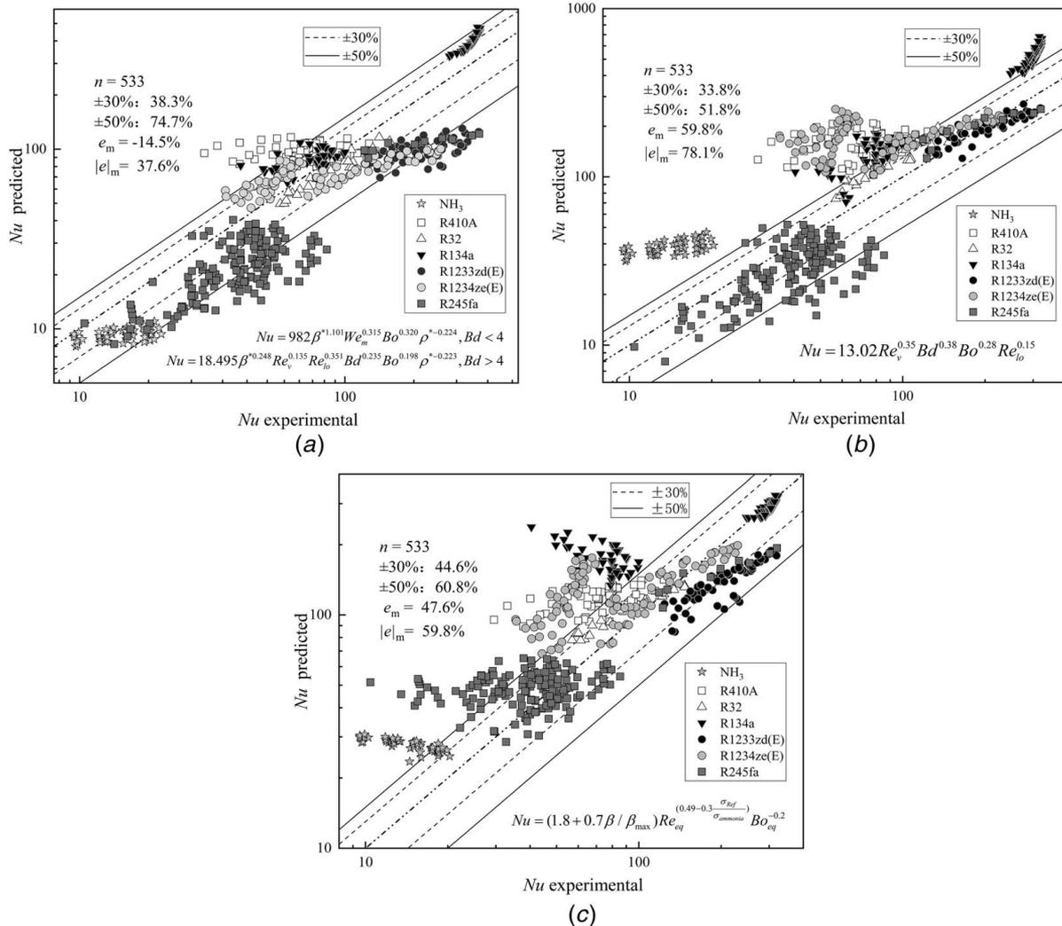
Fig. 4 Predicted Nusselt numbers versus experimental ones. Correlations proposed by: (a) Amalfi et al. [2]; (b) Vakili-Farahani et al. [3]; (c) Ayub et al. [34]. ( $n$ : number of data points,  $e_m$ : mean error =  $\frac{1}{n} \sum ((f_{pre} - f_{ex}) / f_{ex})$ ,  $|e|_m$ : mean absolute error =  $\frac{1}{n} \sum (|(f_{pre} - f_{ex}) / f_{ex}|)$ ).
