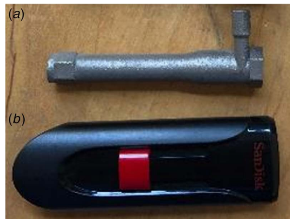
Fig. 3 (a) Additively manufactured vortex tube compared to (b) USB memory stick
