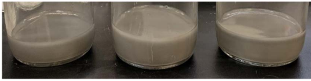
Fig. 3 From left to right: 5% wt., 10% wt., and 20% wt. gallium-in-ethanol emulsions.
