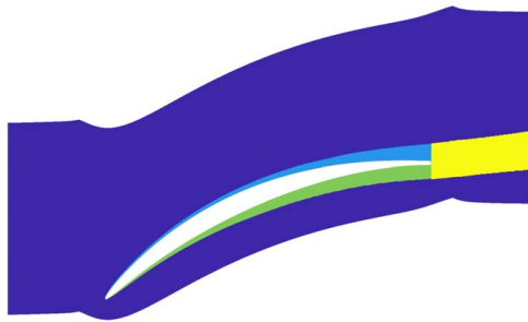
Fig. 5 Example domain decomposition for the NACA65 Tu4 case
