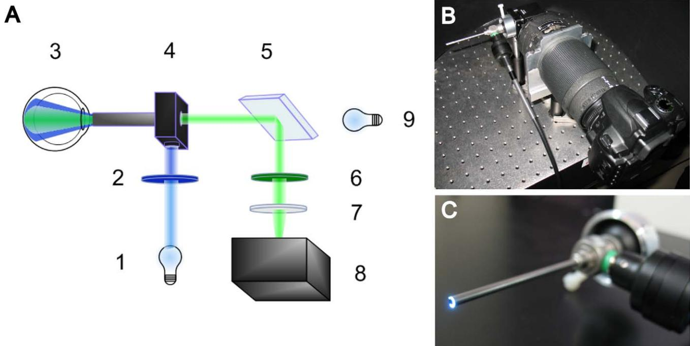
**Figure 1.** (A) System schematic. 1: fluorescent light source, 2: excitation filter, 3: in vivo eye, 4: endoscope, 5: DM/BS, 6: emission filter, 7: lens, 8: CCD, 9: auxiliary light source. (B) Photograph of the setup. (C) Magnification of the endoscope and custom made adaptor.
