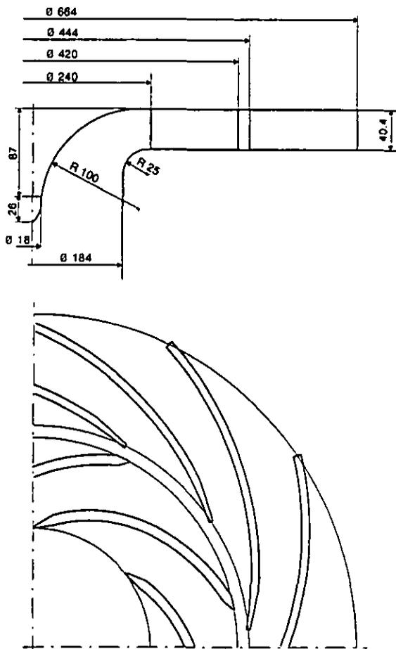
Fig. 2 Impeller and vaned diffuser geometry
