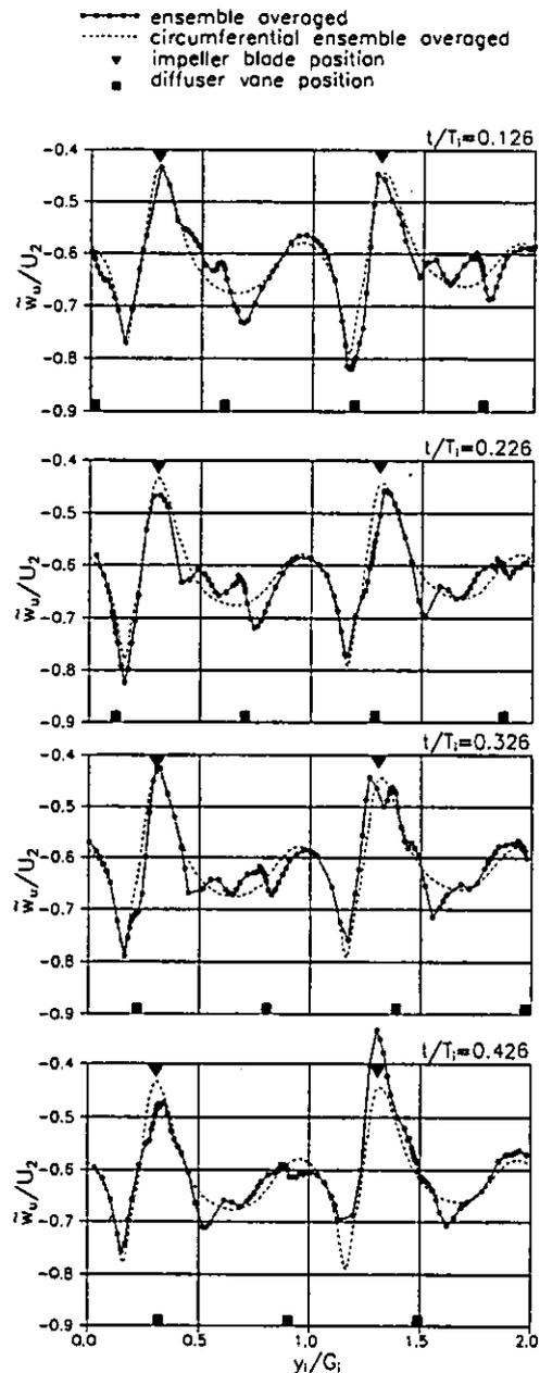
Fig. 8 Instantaneous distributions of the ensemble averaged tangential relative velocity at the impeller outlet, midspan position
