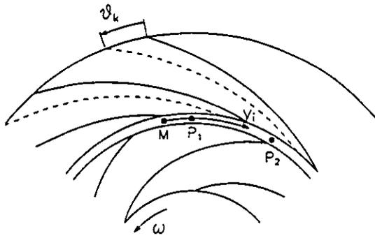
Fig. 3 Sketch of the radial rows of blades and reference coordinates
