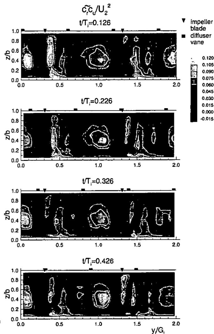
Fig. 10 Instantaneous pictures of the ensemble averaged non dimensional moment of momentum of flow rate at the impeller outlet
