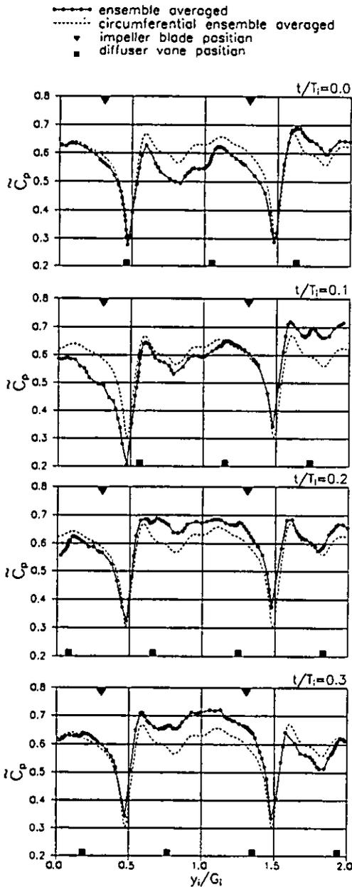
Fig. 11 Instantaneous distributions of the ensemble averaged static pressure coefficient at the impeller outlet
