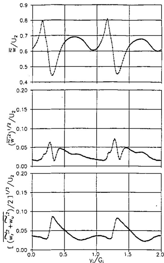
Fig. 5 Circumferential ensemble averaged relative velocity, stator generated unsteadiness and unresolved unsteadiness at the impeller outlet, midspan position
