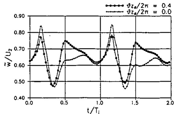
Fig. 4 Ensemble averaged relative velocity distributions for two different circumferential locations of the probe, at the impeller outlet, midspan position
