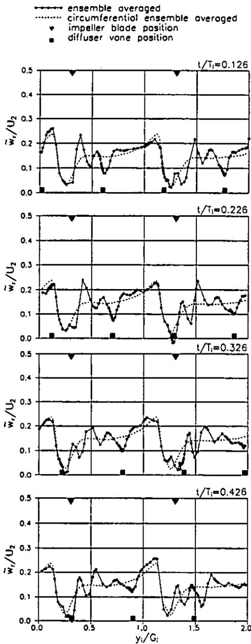
Fig. 7 Instantaneous distributions of the ensemble averaged radial velocity at the impeller outlet, midspan position
