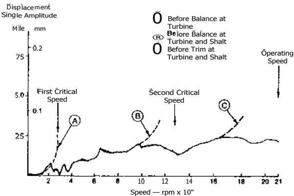
Fig. 2 Results of high-speed balancing T53 power turbine
