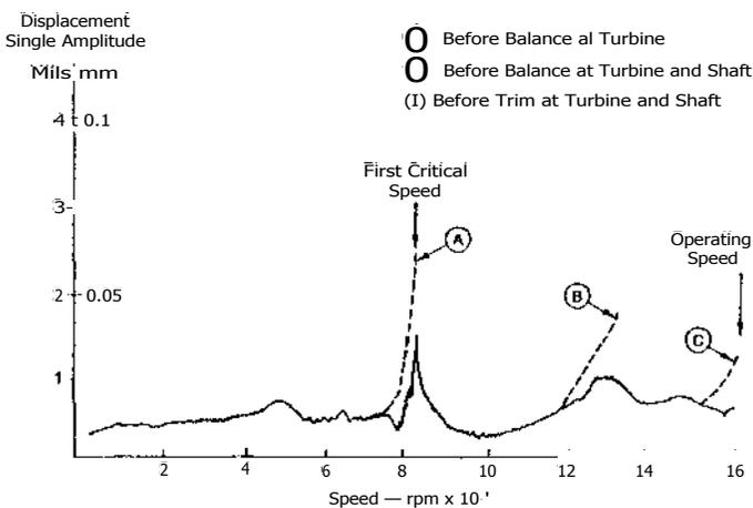
Fig. 3 Results of high-speed balancing T55 power turbine
