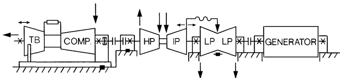
Figure 7. Configuration for Double-Flow Exhaust Turbine.
