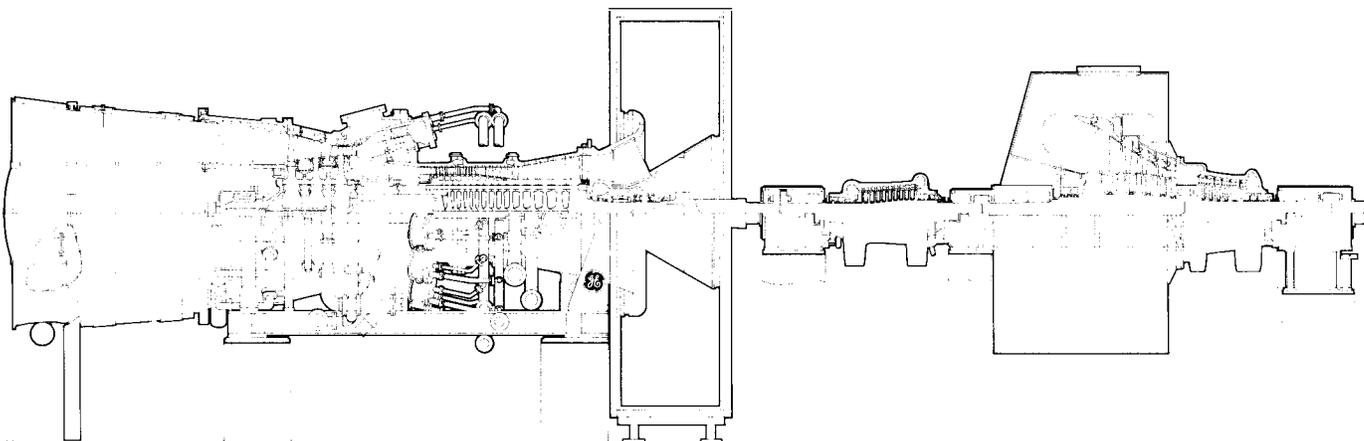
Figure 1. Cross Section of GE Single-Shaft 107F Turbine.
