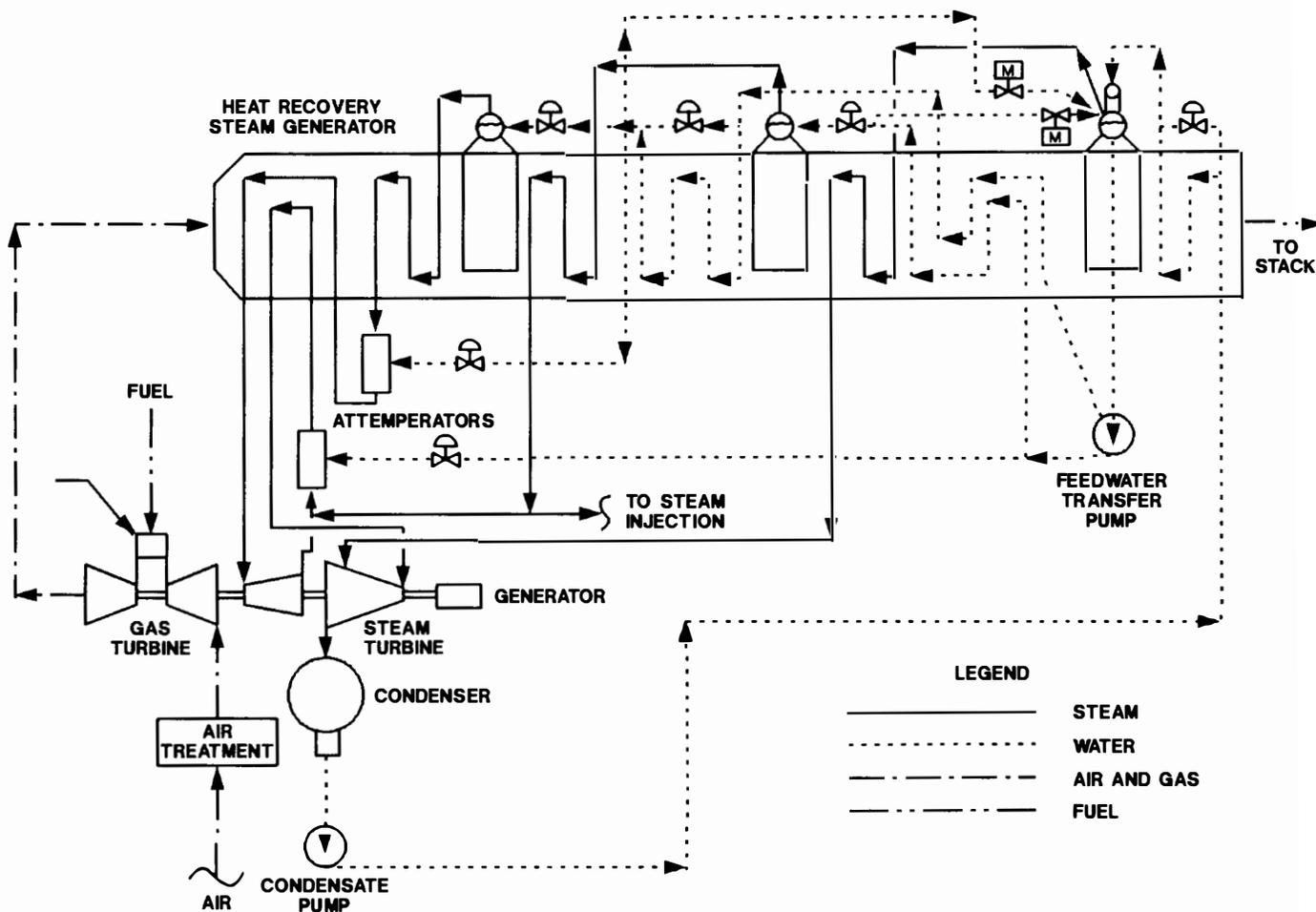
Figure 2. Cycle Schematic.
