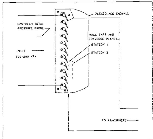
Fig. 2 - Sketch of Cascade Test Section for VPI & SU Transonic Wind Tunnel
