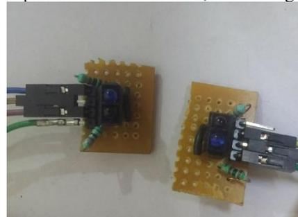
Figure 1: The probes constructed from TCRT 5000 and resistors.
