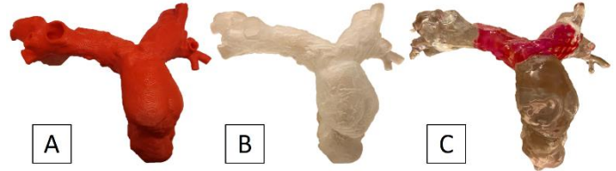
FIGURE 1: 3D PRINTED MODELS FOR PA STENOSIS CASE. (A) HOLLOW PLA, (B) HOLLOW FLEXIBLE PLASTIC, (C) SOLID FIRM PLASTIC WITH EMBEDDED STENT MODELS.
