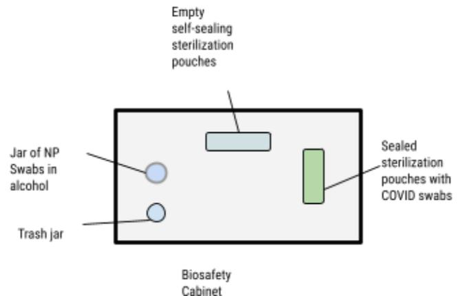
**FIGURE 3:** BIOSAFETY CABINET SET UP.
