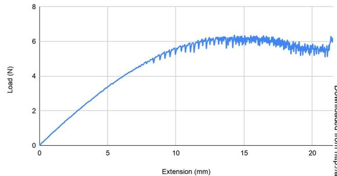
**FIGURE 5: GRAPH OF EXTENSION OF THE SWABS VS LOAD.**
