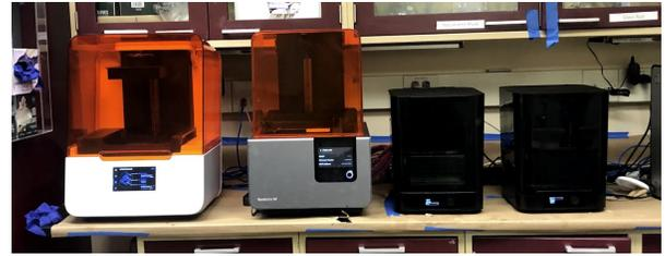
**FIGURE 2:** PRINTING SET UP. FROM LEFT TO RIGHT: FORM 3B PRINTER, FORM 2 PRINTER, FORM WASH, AND FORM CURE.
