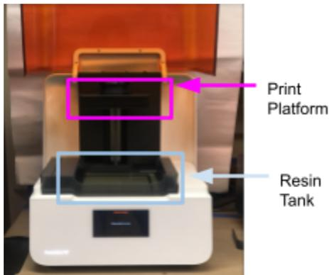
**FIGURE 1:** FORM 3B PRINTER AND ITS COMPONENTS.
