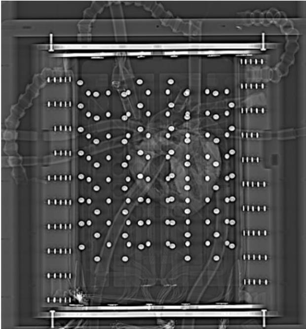
**FIGURE 9:** A CT scan of a previously reanimated human heart positioned in the epicardial mapping tank with all 252 electrodes.
