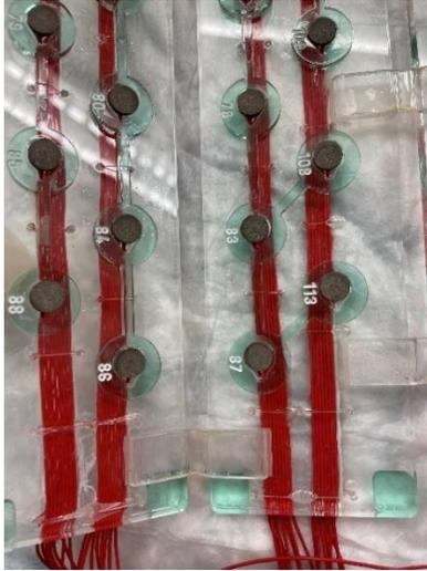
**FIGURE 5:** The bottom electrode plate composed of thin acrylic sheets connected by flexible hinges.
