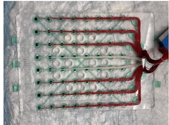
**FIGURE 4:** Top plate of electrodes from the epicardial mapping tank. Holes in the acrylic allow direct access to the anterior surface of the heart.
