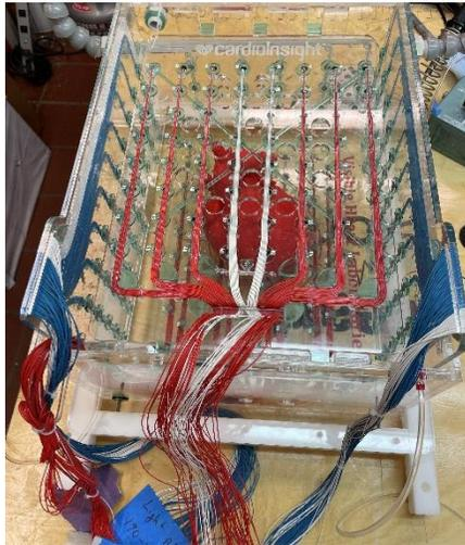
**FIGURE 6:** The completed epicardial mapping tank with all 252 electrodes, shown with a 3D printed heart.
