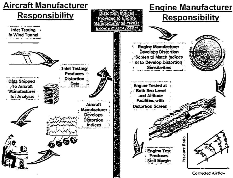
Fig. 1 – Current Inlet-Engine Integration Test Methodology
