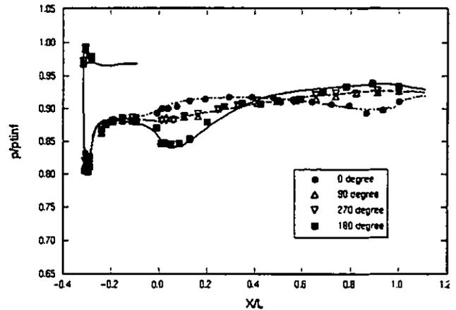
Fig. 9 – Axial Pressure Distribution – S-Duct
