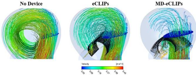
**Figure 3:** Side view of velocity vectors at the symmetry plane for eCLIPs, eCLIPs-MD and no device (ND) at peak systole
