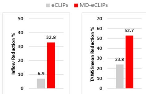
**Figure 5:** Aneurysm inflow and time-averaged aneurysm WSS reductions for the eCLIPs and MD-eCLIPs over no device case
