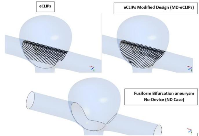
**Figure 2:** Geometry of the fusiform bifurcation aneurysm with the eCLIPs and eCLIPs-Modified Design implanted at the neck
