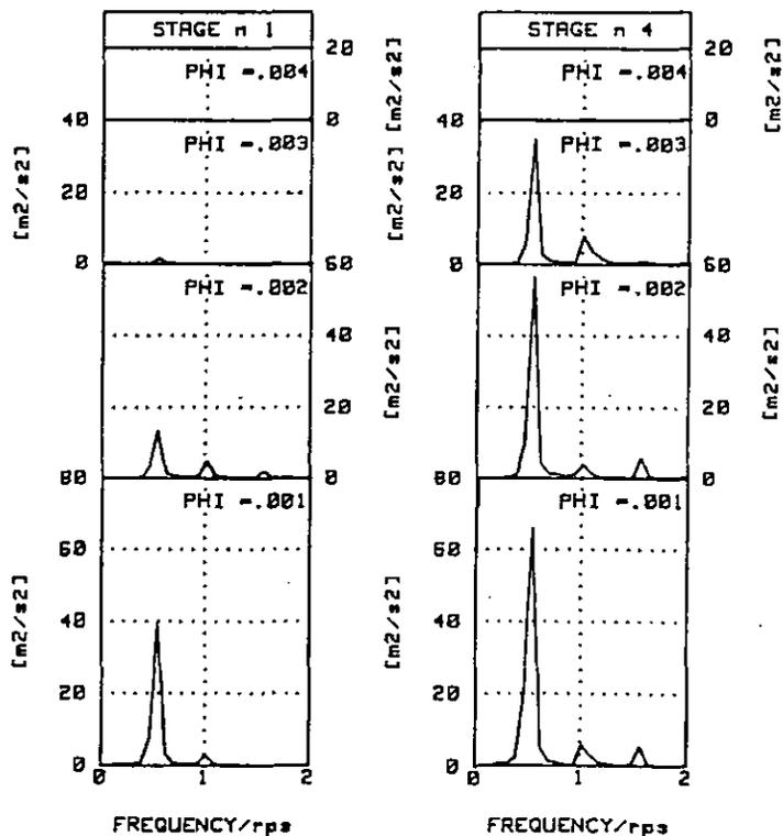
Fig. 11 - Power spectra of the velocity at the impellers exit ( $x/b=0.5$ ).
