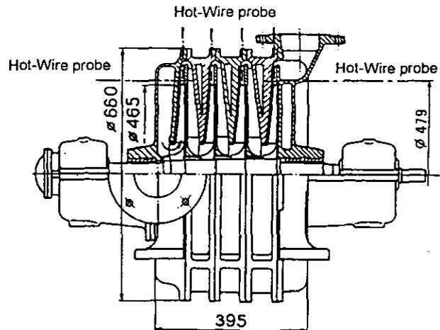
Fig. 1 - Test blower and measuring sections.
