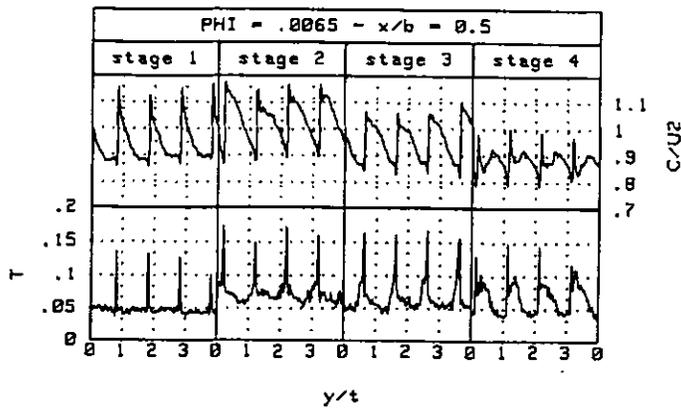
Fig. 7 - Blade to blade profiles of flow parameters at  $x/b=0.5$ : comparison among the four stages at nominal conditions ( $\varphi=0.0065$ ).
