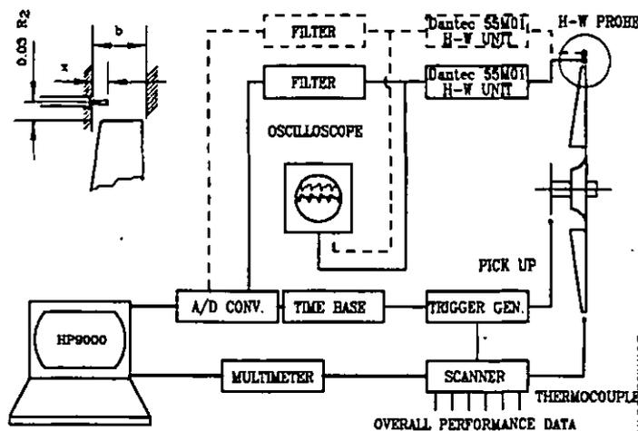
Fig. 3 - Schematic of experimental rig.
