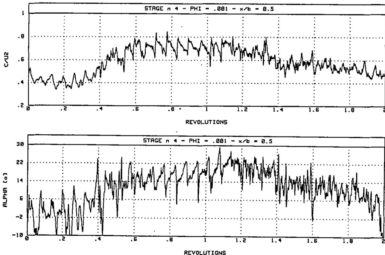
Fig. 12 - Absolute velocity and flow angle traces at the fourth impeller exit at  $x/b=0.5$  at unsteady flow condition ( $\varphi=0.0010$ ).
