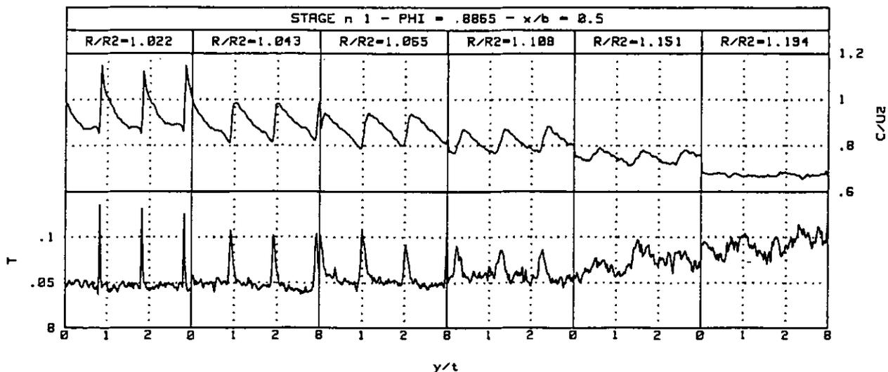
Fig. 8 - Flow parameters traces in the first stage diffuser at  $x/b=0.5$ : comparison among differing radial position, at nominal conditions ( $\varphi=0.0065$ ).
