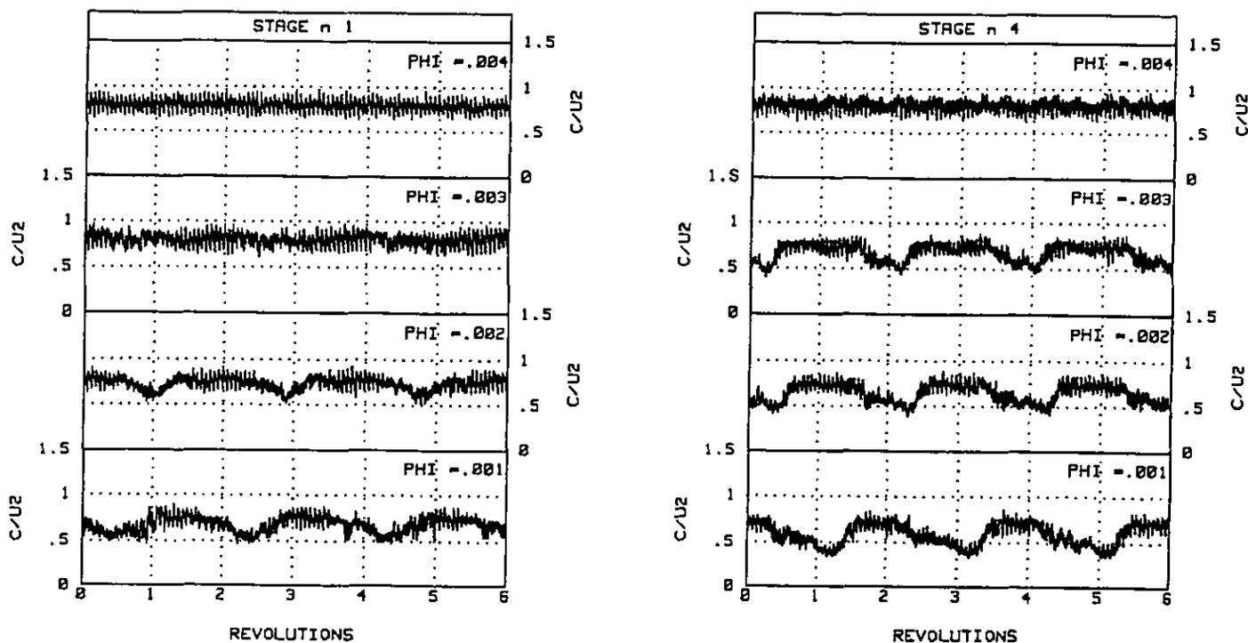
Fig. 10 - Velocity traces at the impellers exit in unsteady flow conditions ( $x/b=0.5$ ).
