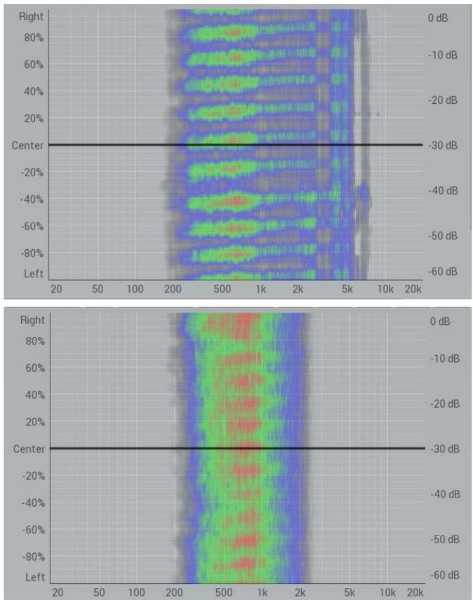
**FIGURE 4. Spectrograph Comparison.** **Top.** A spectrograph of an audio recording of the carotid artery from our improved vascular Doppler. The vertical and horizontal axis corresponds to time and frequency in Hertz respectively and the colors correlate to magnitude at the respective frequency and time. **Bottom.** A spectrograph of an audio recording of the carotid artery from a Parks Medical Model 811-B vascular Doppler currently in use at the University of Minnesota’s MHealth Hospital.
