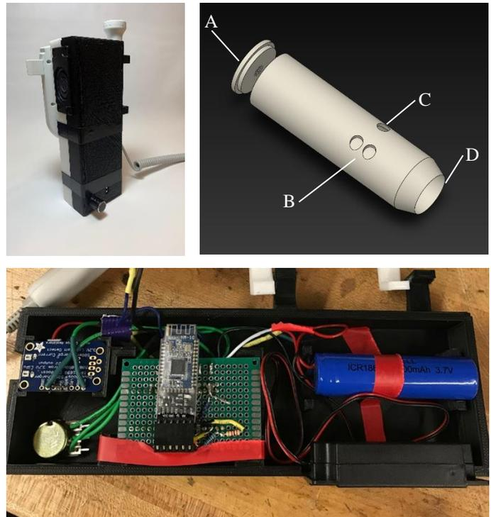
**FIGURE 2. Vascular Doppler Prototype.** Top Left: The current prototype of the improved vascular Doppler. Top Right: A Computer-Aided-Design Model of the next design of the vascular Doppler with parts labeled: A) speaker, B) volume adjustment controls, C) power control, and D) transducer. Bottom: Electronic components consolidated and soldered in a 3-D printed housing.
