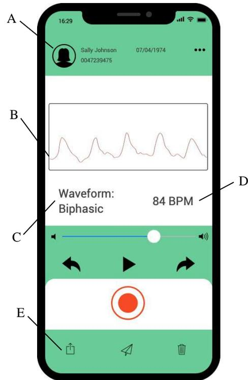
**FIGURE 3. Mobile Application Mock-Up.** The mobile application would serve as a companion to the BLE-enabled Doppler device and include A) patient summary, B) Doppler waveform display, C) automated waveform interpretation, D) heart rate, E) means to save the Doppler data to the patient's electronic medical record.
