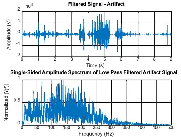
Fig. 5: (Top) Plot of filtered artifact sound signal; (Bottom) Normalized power spectrum of the filtered artifact sound signal
