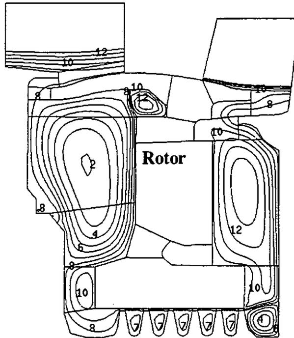
Figure 2 Stream Function Distribution inside the Stage 1-2 Cavities.
