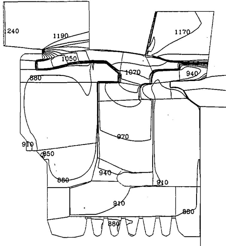
Figure 4 Static Temperature Distribution inside the Stage 1-2 Cavities and the Central Support Wall.
