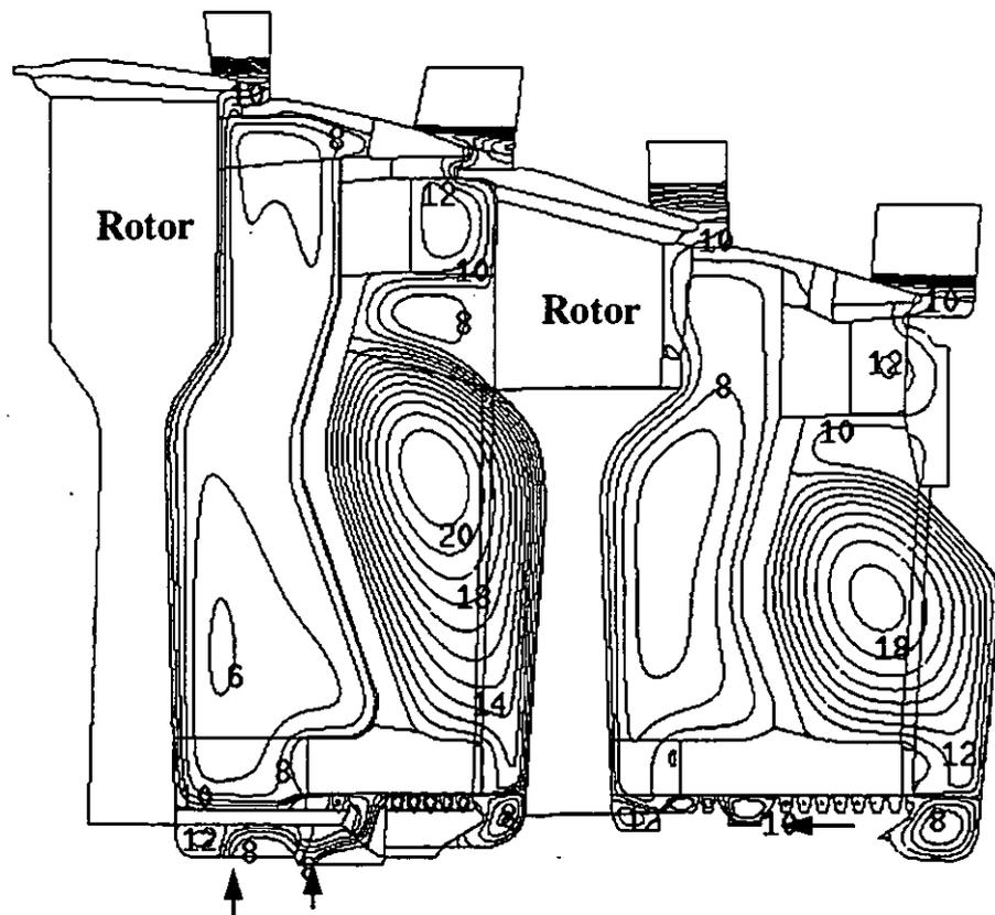
Figure 3 Stream Function Distribution inside the Stages 2-3 and 3-4 Cavities.
