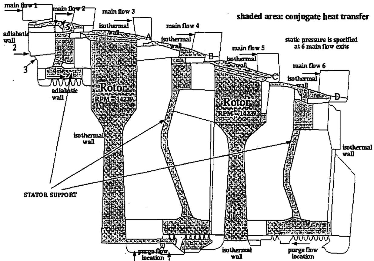
**Figure 1. Flow Model for the Allison T-56/501D Turbine Cavities**
