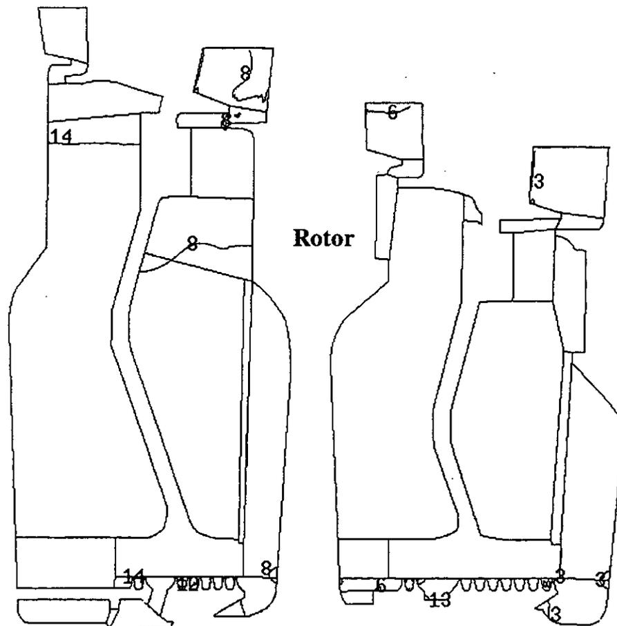
Figure 7 Static Pressure Distribution inside the Stages 2-3 and 3-4 Cavities.
