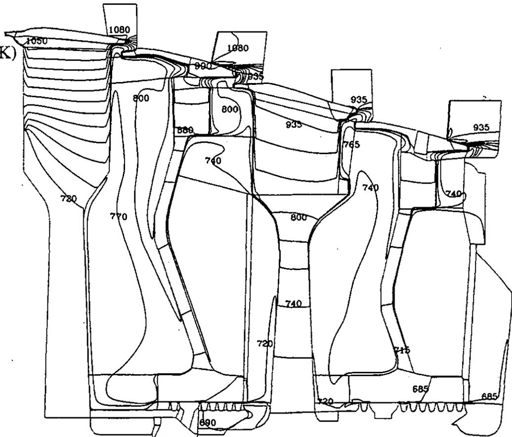
Figure 5 Static Temperature Distribution inside the Stages 2-3 and 3-4 Cavities, the Central Support Walls and the Rotors Support Walls.
