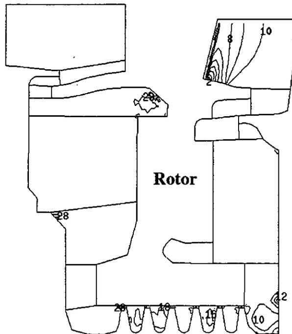
Figure 6 Static Pressure Distribution inside the Stage 1-2 Cavities.
