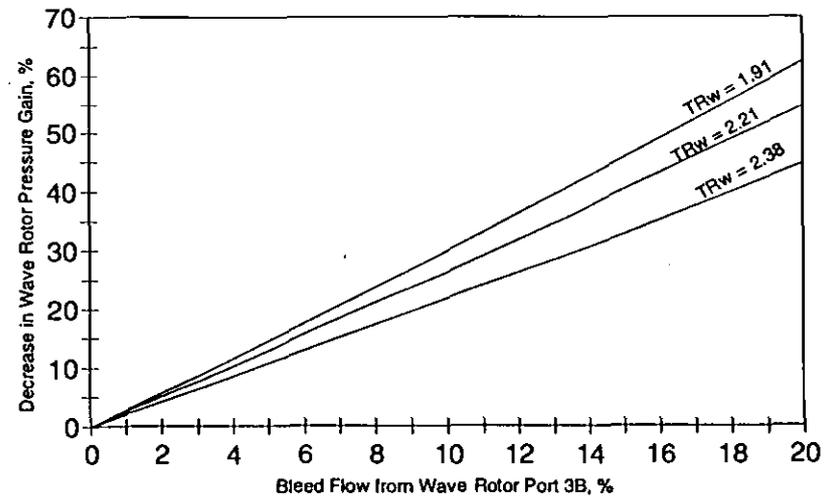
Figure 4: Decrease in Wave Rotor Pressure Gain as a Function of Bleed
