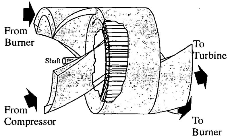
Figure 1: Four-port Wave Rotor Schematic Diagram
