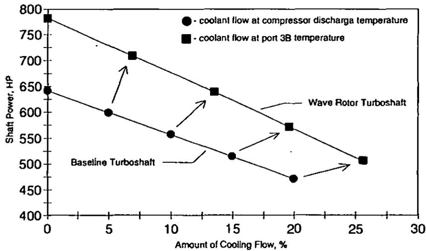
Figure 7: Design Point Shaft Power for Baseline and Wave Rotor-Topped Turboshfts as a Function of Required Cooling Flow
