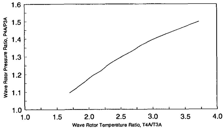
Figure 3: Design Point Wave Rotor Pressure Ratio
