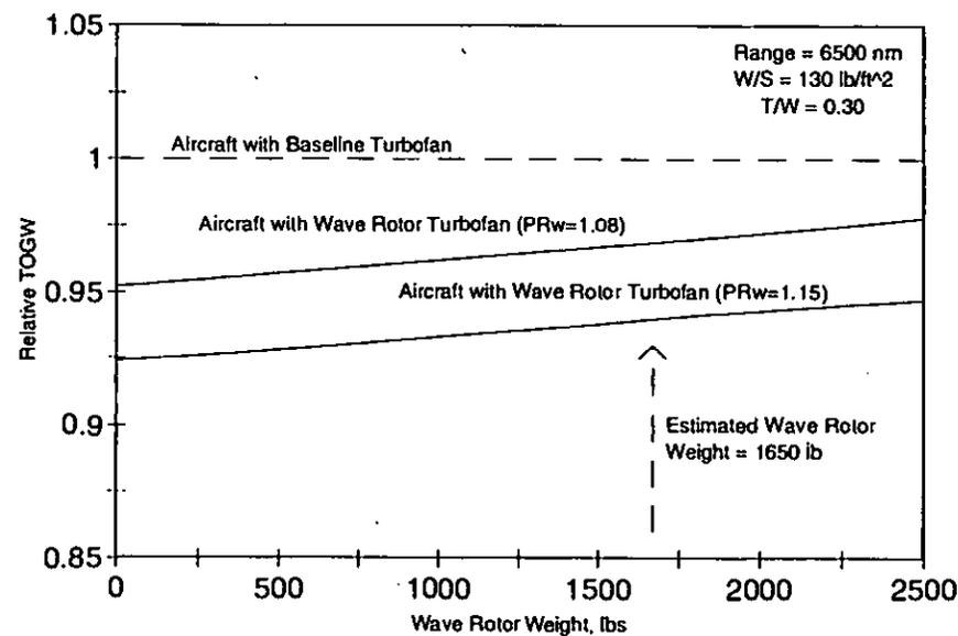
Figure 11: TOGW Benefit for a Subsonic Transport with a Wave Rotor-Topped Turbofan
