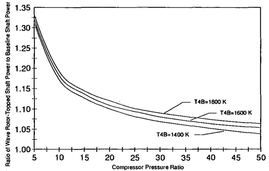
Figure 6: Wave Rotor Shaft Power Benefit for Turboshfts of Varying CPR and T4B
