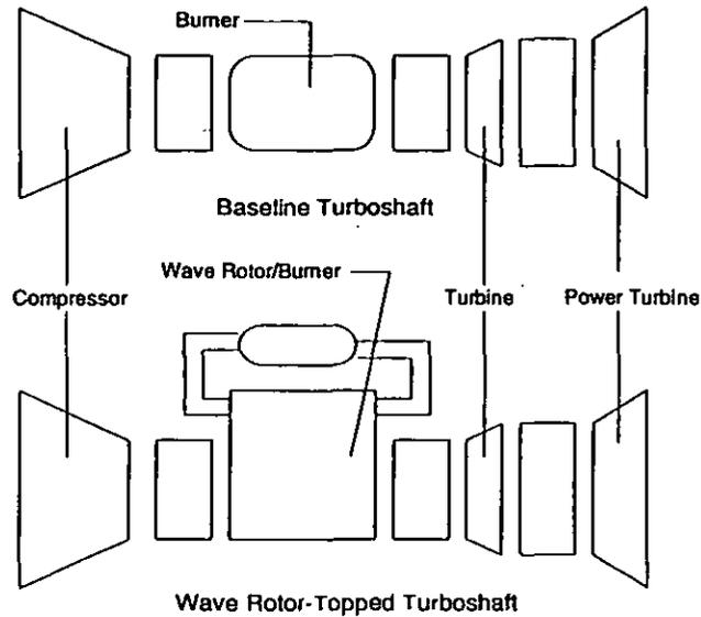
Figure 5: Baseline and Wave Rotor-Topped Turboshaft Schematic Diagrams
