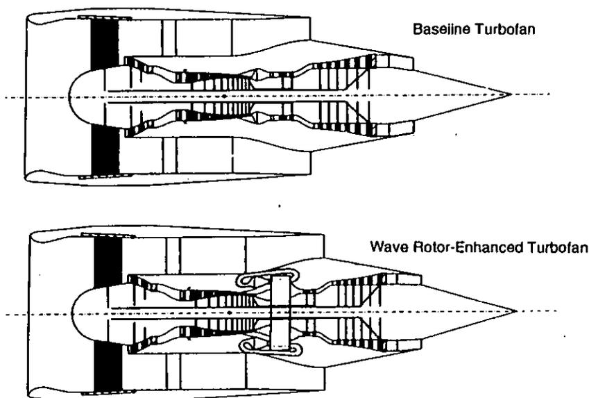
Figure 10: Baseline and Wave Rotor-Topped Turbofan Schematic Diagrams
