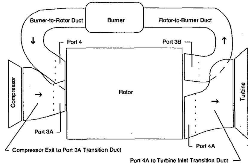
Figure 2: Wave Rotor and Burner Schematic Diagram
