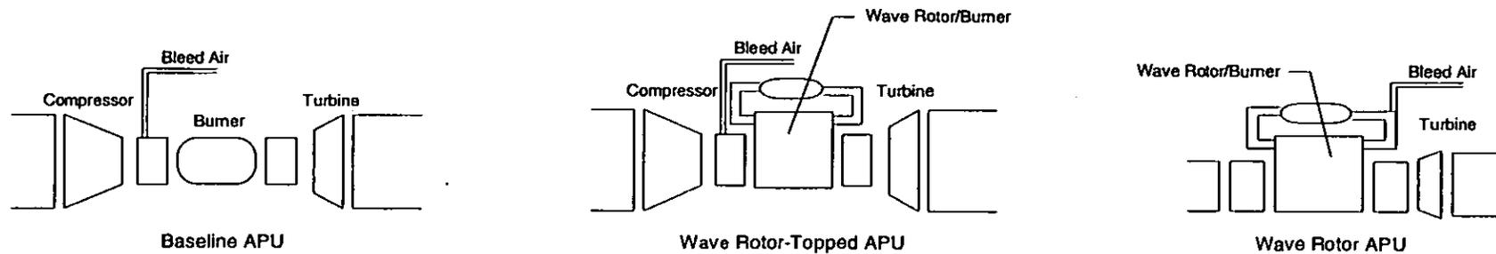
Figure 9: Auxiliary Power Unit Schematic Diagrams
