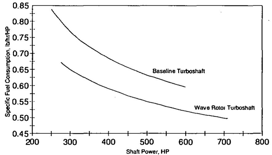
Figure 8: Off-Design Performance Benefit for Wave Rotor-Topped Turboshft Engine
