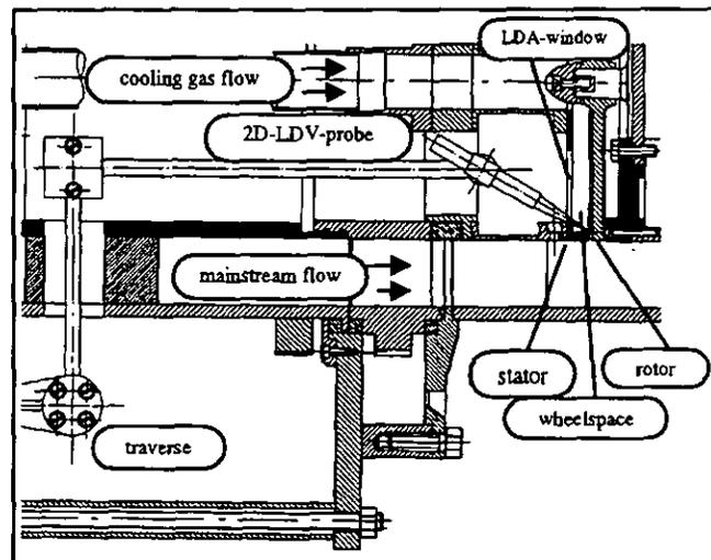
FIG. 6: DETAILS OF THE 2D-LDA-MEASUREMENTS INTO THE MACHINE
