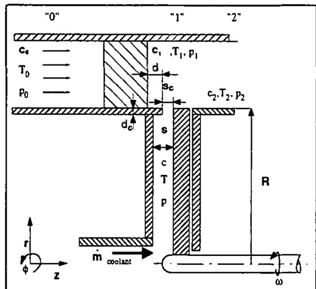
FIG. 4: CONFIGURATION 2 IS COMPOSED OF A STATOR WITH RIM SEAL COMBINED WITH A PLANE ROTOR DISC
