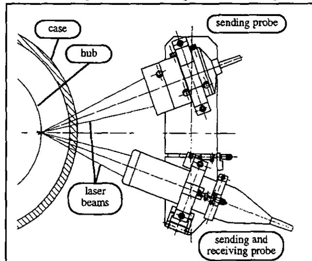
FIG. 5: QUASI 3D-LDA-MEASUREMENTS IN THE COOLANT-MAINSTREAM INTERACTION REGION
