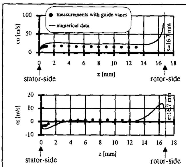
FIG. 18: CIRCUMFERENTIAL VELOCITY COMPONENT
