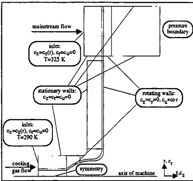
FIG. 14: COMPUTED DOMAIN OF THE WHEELSPACE WITH MAINSTREAM
