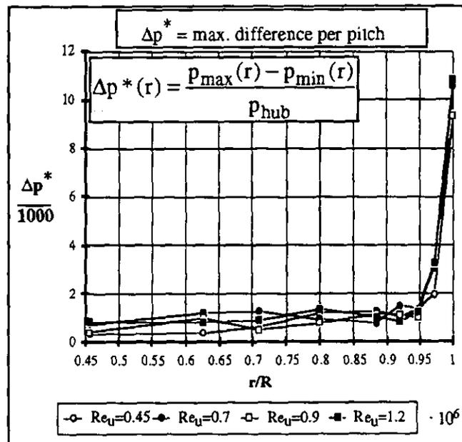
FIG. 11: MAXIMUM PRESSURE DIFFERENCE FOR CONFIGURATION 1  $c_w = 6500, s = 1.7$  mm,  $Re_{c1} = 0.74 \cdot 10^6$
