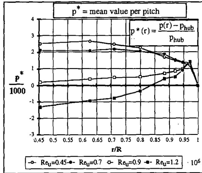
FIG. 10: NONDIMENSIONAL PRESSURE FOR CONFIGURATION 1  $c_w = 6500, s = 1.7$  mm,  $Re_{c1} = 0.74 \cdot 10^6$
