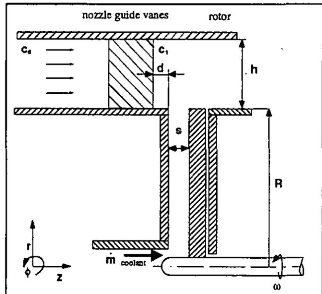
FIG. 3: CONFIGURATION 1 IS COMPOSED OF A PLANE STATOR COMBINED WITH A PLANE ROTOR DISC
