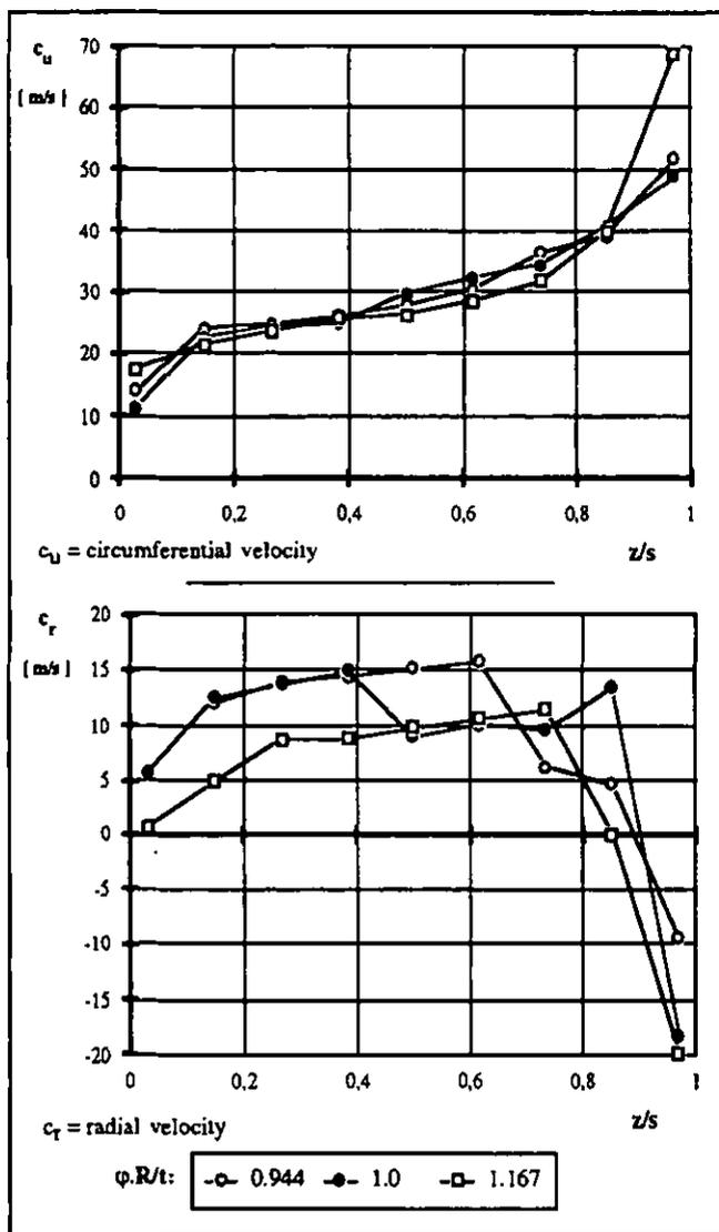
FIG. 12: CIRCUMFERENTIAL AND RADIAL VELOCITY IN THE WHEELSPACE WITH GUIDE VANES, CONF. 1
