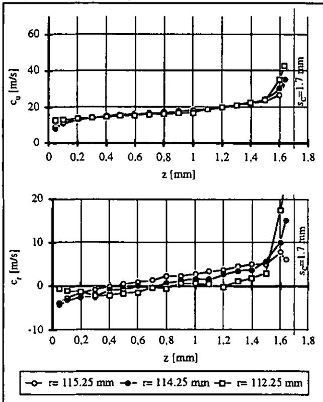
FIG. 7: CIRCUMFERENTIAL AND RADIAL VELOCITY IN THE WHEELSPACE NEAR THE RIM SEAL WITHOUT VANES, CONF.2,
