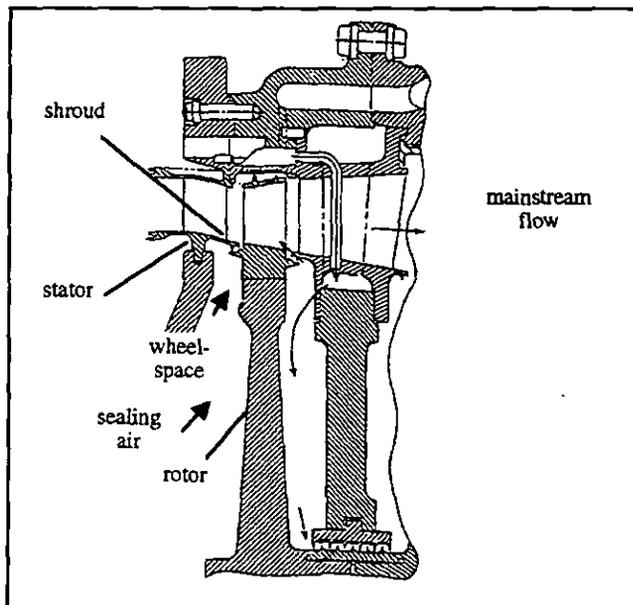
FIG. 1: WHEELSPACE IN A TURBINE ROTOR
