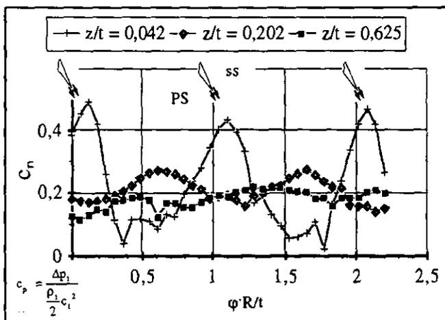
FIG. 9: PRESSURE COEFFICIENT AT DIFFERENT POSITIONS DOWNSTREAM OF THE TRAILING EDGE OF NOZZLE GUIDE VANES ( $Ma_{c1} = 0.787$ ;  $Re_{c1} = 1.9 \cdot 10^6$ )
