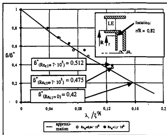
FIG. 13: THE VARIATION OF THE RELATIVE ROTATION OF THE CORE WITH RADIAL OUTFLOW AND MAINSTREAM FLOW WITH GUIDE VANES, CONF.2,  $G_c=0.005$
