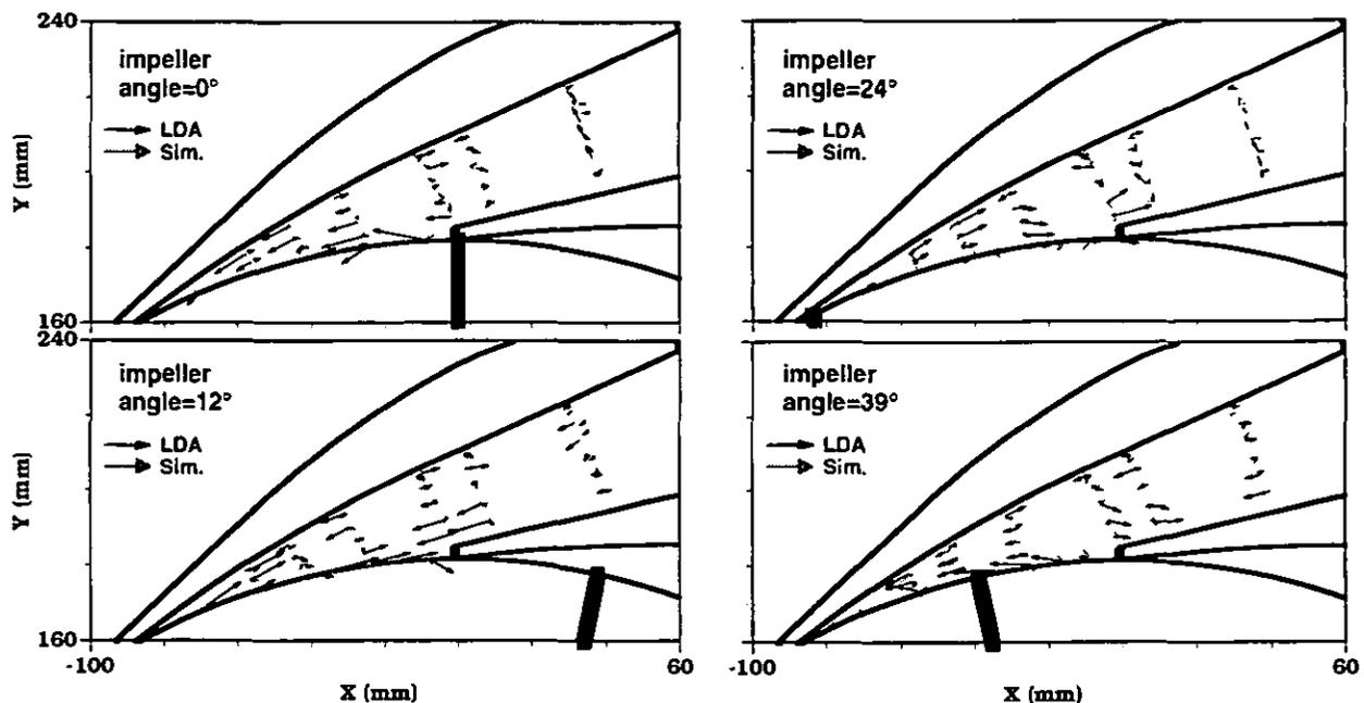
Fig. 8B Measured and calculated fluctuations in velocity vectors (unsteady - time average) at 4 impeller positions
