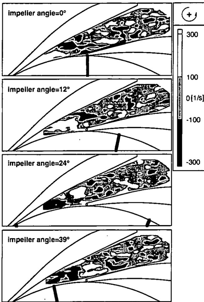
**Fig. 12 Measured fluctuation in vorticity at 4 impeller positions**
