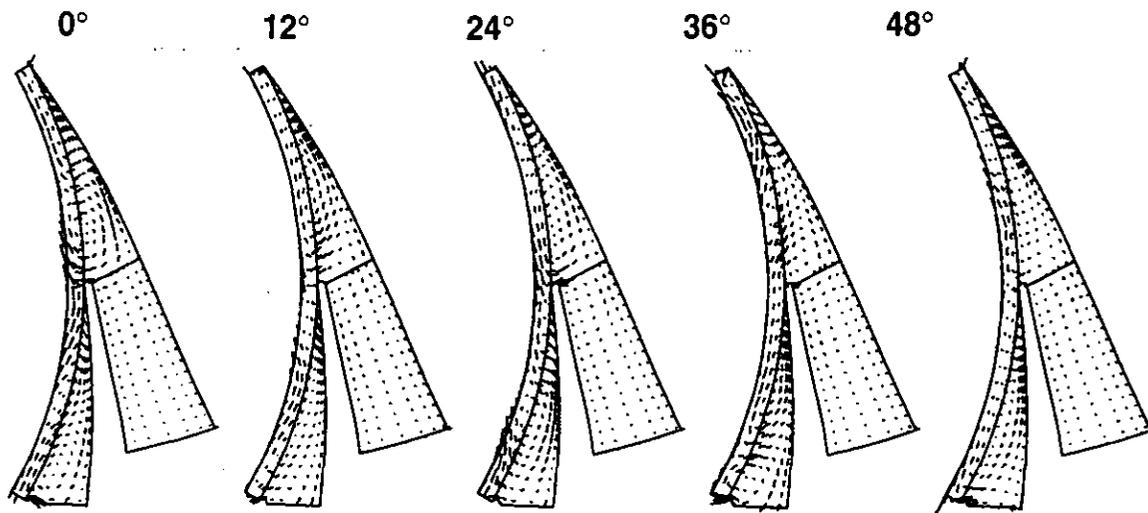
Fig. 8A Fluctuations in velocity vectors (unsteady - time average) at impeller positions 0°, 12°, 24°, 36°, 48°
