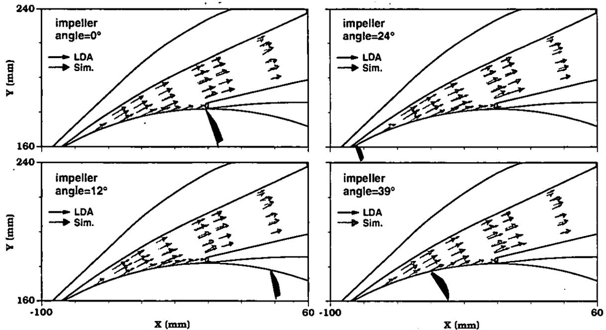
Fig. 9 Measured and calculated velocity vectors at 4 impeller positions
