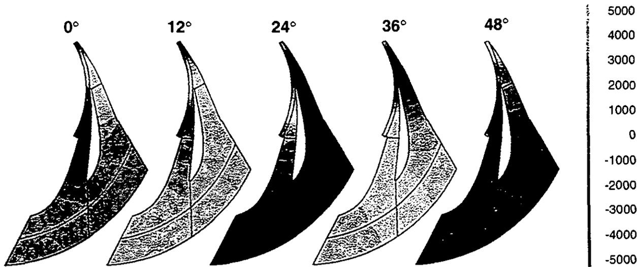
Fig. 5 Fluctuations in static pressure  $P$  (unsteady - time average,  $N/m^2$ ) at impeller positions  $0^\circ$ ,  $12^\circ$ ,  $24^\circ$ ,  $36^\circ$ ,  $48^\circ$
