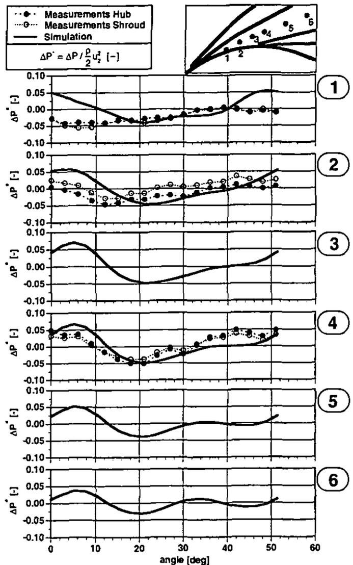
Fig. 11 Measured and calculated pressure along the diffuser center line
