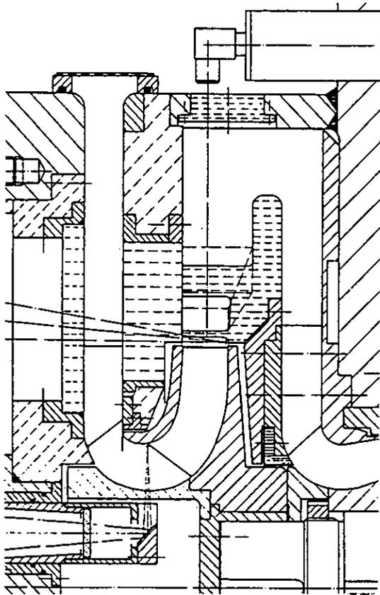
Fig. 1 Test pump with vaned diffuser
