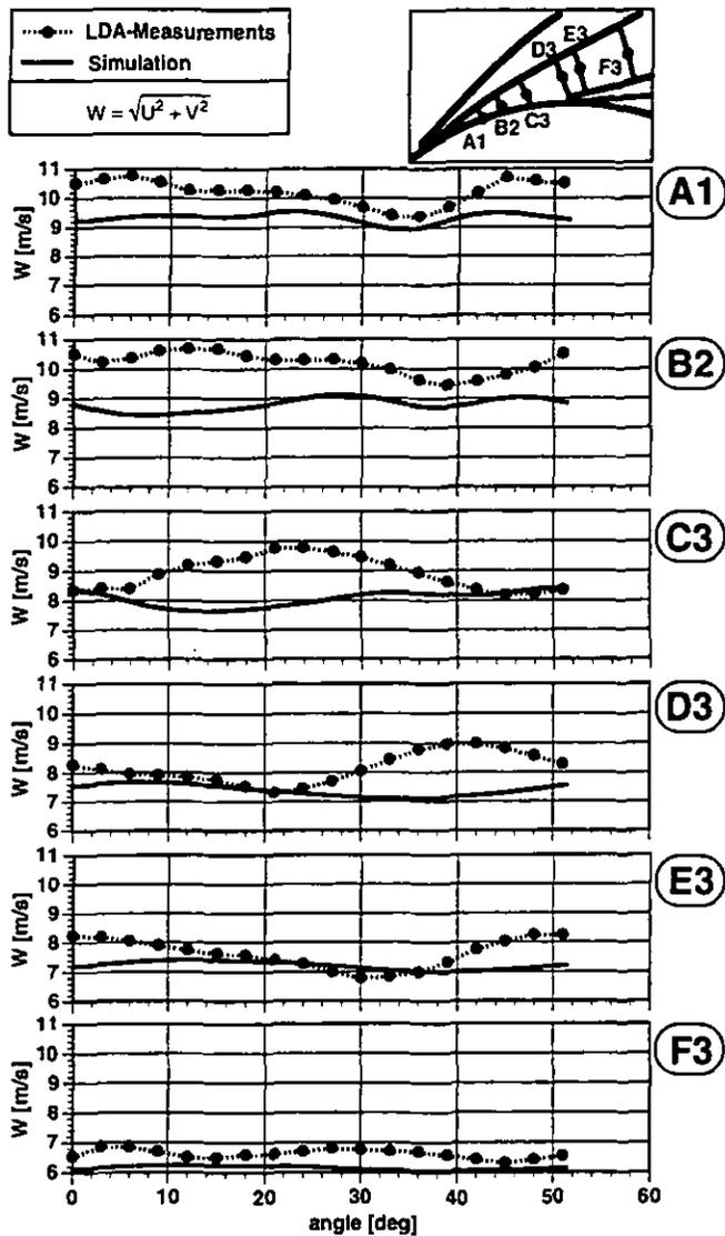
Fig. 10 Measured and calculated velocity level  $w$  along the diffuser center line
