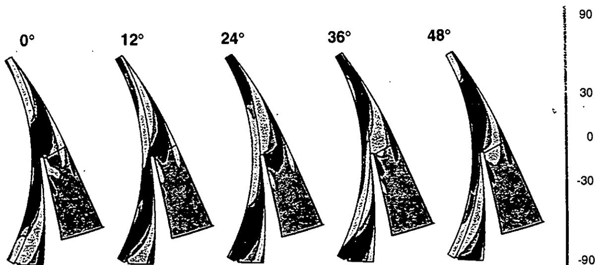
Fig. 7 Fluctuations in vorticity (unsteady - time average, 1/s) at impeller positions  $0^\circ$ ,  $12^\circ$ ,  $24^\circ$ ,  $36^\circ$ ,  $48^\circ$
