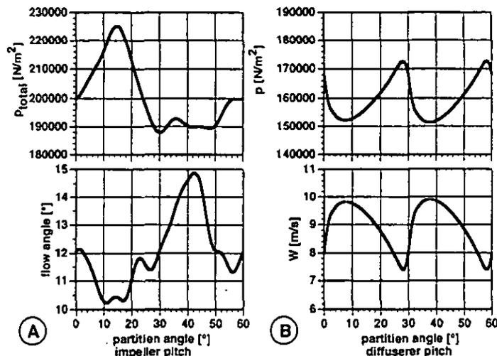
Fig. 3 Inlet boundary conditions for the simulation: A) Time periodic total pressure profile and flow angle B) Resulting time-averaged static pressure and velocity profile
