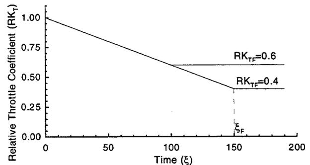
FIG.4 THROTTLE CLOSURE PROCESS
