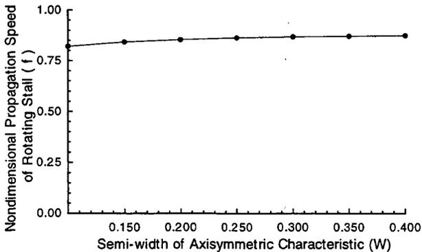
FIG.24 THE EFFECT OF W ON THE PROPAGATION SPEED OF ROTATING STALL
