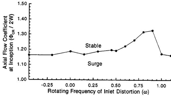
FIG.18 THE EFFECT OF ROTATING SPEED OF INLET DISTORTION ON FLOW COEFFICIENT AT INCEPTION POINT OF SURGE FOR  $B=2.6$
