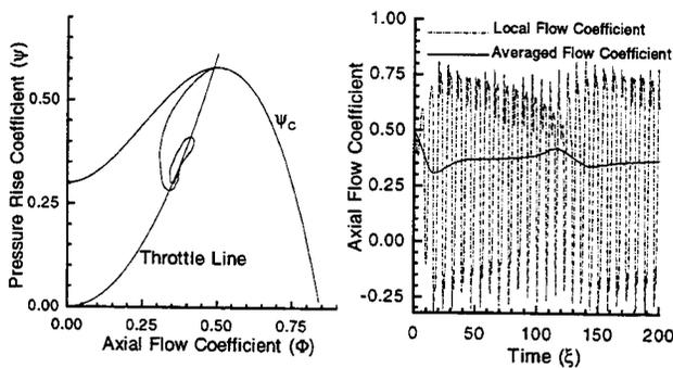
FIG.10 THE POST STALL TRANSIENTS FOR THE SAME CASE AS FIG.5, EXCEPT  $DA=0.1$  AND  $\omega=0.80$
