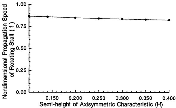
FIG.23 THE EFFECT OF H ON THE PROPAGATION SPEED OF ROTATING STALL
