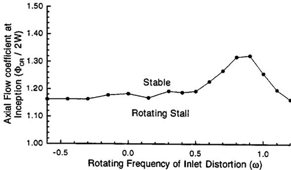
FIG.14 THE EFFECT OF ROTATING SPEED OF INLET DISTORTION ON FLOW COEFFICIENT AT INCEPTION OF ROTATING STALL FOR THE BASE CASE
