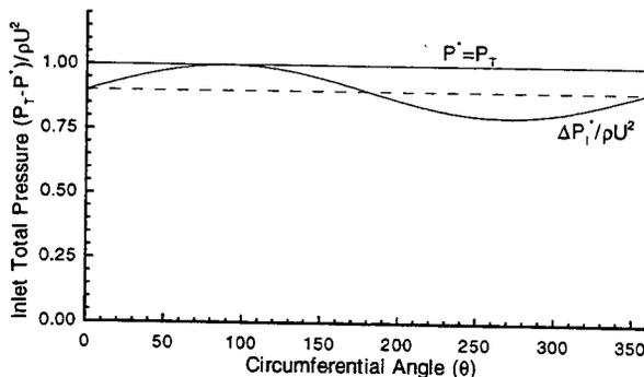
FIG.3 INLET TOTAL PRESSURE PROFILE
