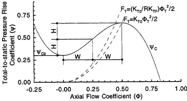
FIG.2 AXISYMMETRIC COMPRESSOR CHARACTERISTIC AND THROTTLE LINE
