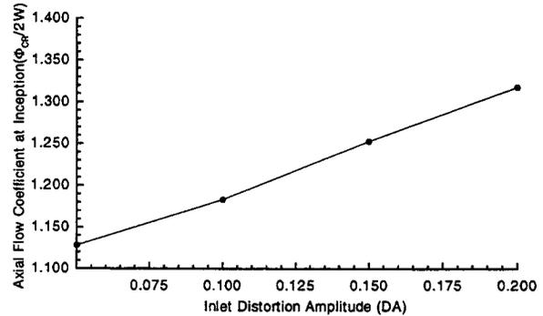
FIG.12 THE EFFECT OF INLET DISTORTION AMPLITUDE ON STALL INCEPTION FLOW COEFFICIENT FOR THE BASE CASE
