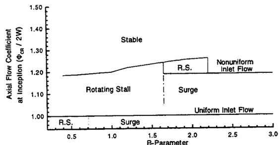
FIG.17 THE EFFECT OF PARAMETER B ON STALL FLOW COEFFICIENT AND INSTABILITY MODE
