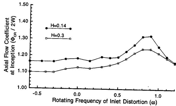
FIG.25 THE EFFECT OF H ON THE RESONANT RESPONSE FREQUENCY
