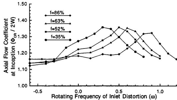
FIG.16 THE EFFECT OF  $f$  ON THE RESONANT RESPONSE FREQUENCY
