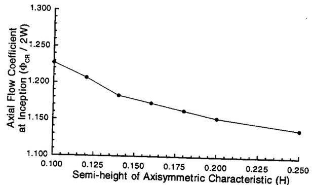
FIG.21 THE EFFECT OF SEMI-HEIGHT ( $H$ ) OF COMPRESSOR CHARACTERISTIC ON STALL FLOW COEFFICIENT
