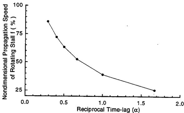
FIG.15 THE EFFECT OF  $\alpha$  ON THE NONDIMENSIONAL PROPAGATION SPEED OF ROTATING STALL
