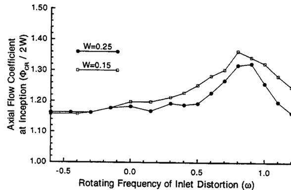
FIG.26 THE EFFECT OF W ON THE RESONANT RESPONSE FREQUENCY
