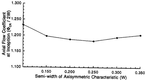
FIG.22 THE EFFECT OF SEMI-WIDTH (W) OF COMPRESSOR CHARACTERISTIC ON STALL FLOW COEFFICIENT
