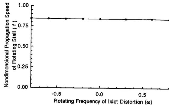
FIG.8 THE EFFECT OF ROTATING SPEED OF INLET DISTORTION ON THE PROPAGATION SPEED OF ROTATING STALL
