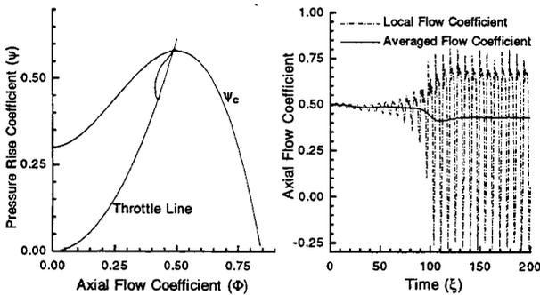
FIG.5 THE POST STALL TRANSIENTS WITH UNIFORM INLET FLOW ( $DA=0.0$ )
