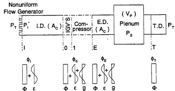
FIG. 1 SKETCH OF THE COMPRESSION SYSTEM AND NOTATIONS
