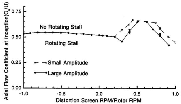
FIG.13 THE EFFECT OF DISTORTION ROTATION RATE ON COMPRESSOR STALL ONSET (Ludwig et al., 1973)
