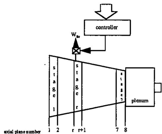
Fig 1 Active surge control using a single-actuator
