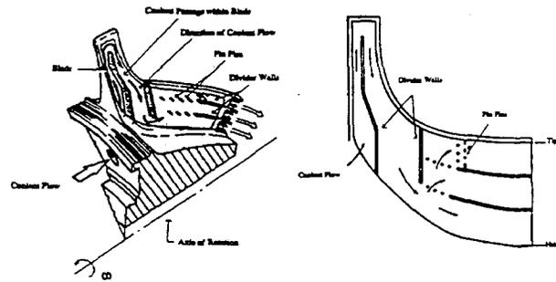
FIGURE 1: SCHEMATIC OF TURBINE BLADE WITH A COOLING PASSAGE INSIDE OF IT
