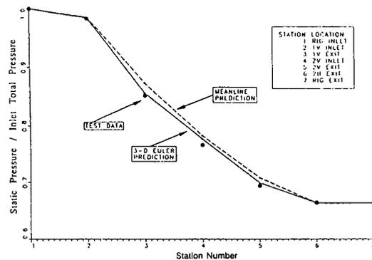
FIG. 10 STATIC PRESSURE DROP THROUGH TURBINE WITH MEAN LINE AND 3-D EULER PREDICTIONS
