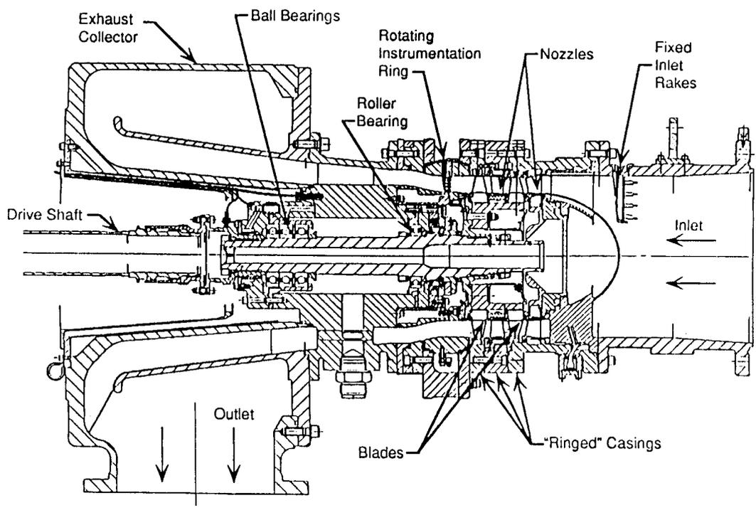
FIG. 2 CROSS SECTION OF TTA
