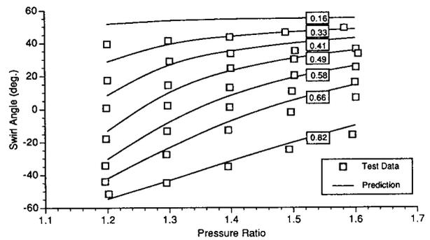
FIG. 8 TURBINE EXIT SWIRL ANGLE VERSUS PRESSURE RATIO FOR THE ATD MODEL WITH CONSTANT LINES OF SPEED PARAMETER
