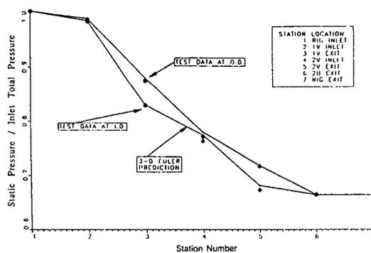
FIG. 11 INNER AND OUTER DIAMETER STATIC PRESSURE MEASUREMENTS WITH 3-D EULER PREDICTION
