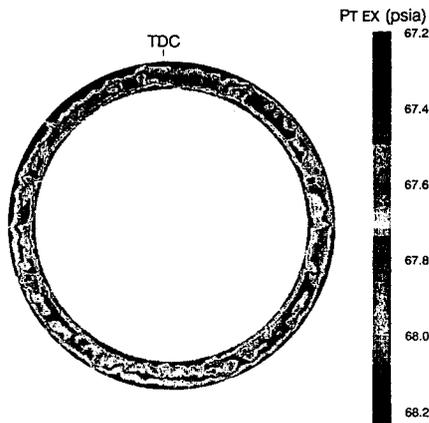
FIG. 5 EXIT PRESSURE PROFILE AT DESIGN POINT (view is aft looking upstream)
