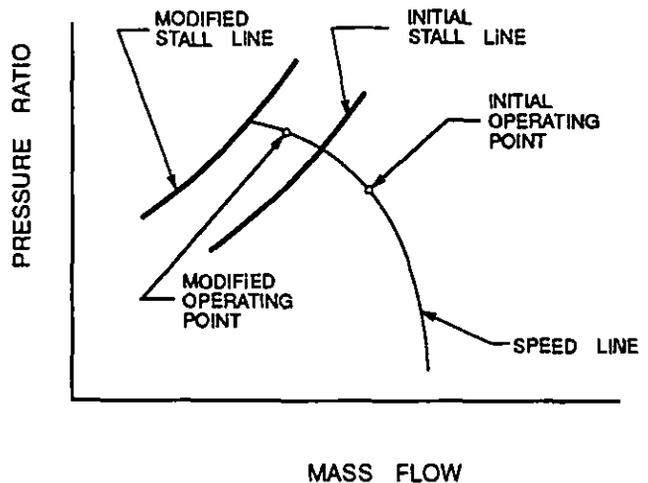
Figure 1. Extending Compressor Operating Range
