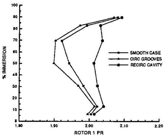
Figure 8. 85% Speed Near-Stall Pressure Ratio Profile
