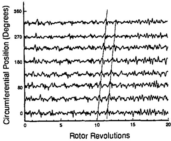
Figure 11. 68% Speed Pre-Stall Operating Point
