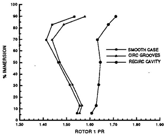
Figure 7. 68% Speed Near-Stall Pressure Ratio Profile
