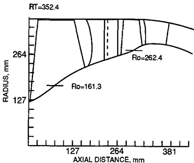
Figure 2. Meridional View of Test Compressor
