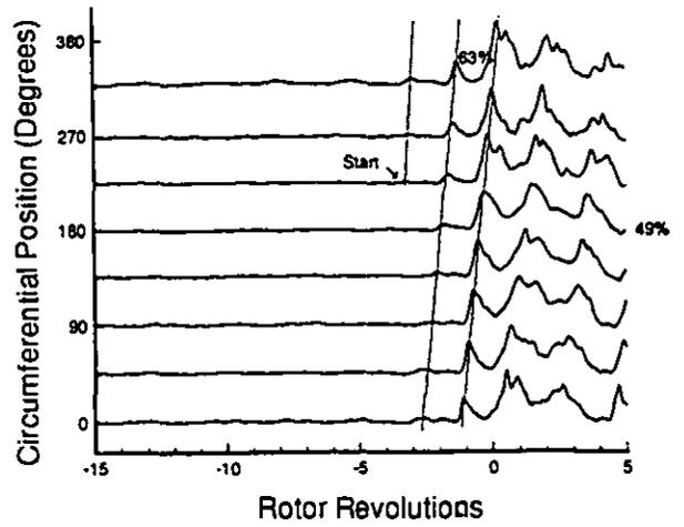
Figure 14. Stall Inception at 98.6% Speed Recirc Cavity
