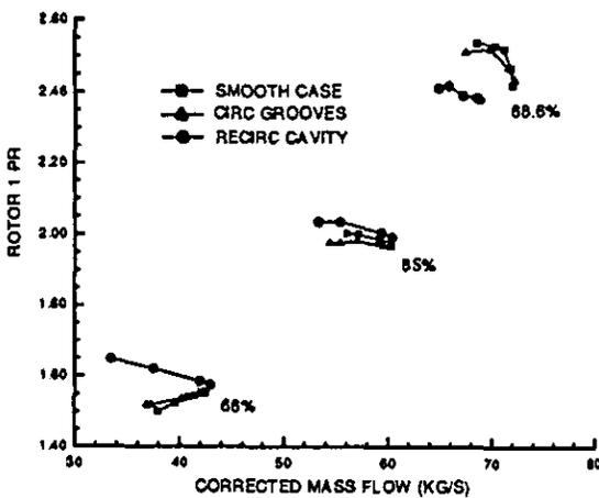
Figure 5. Rotor 1 Pressure Characteristic
