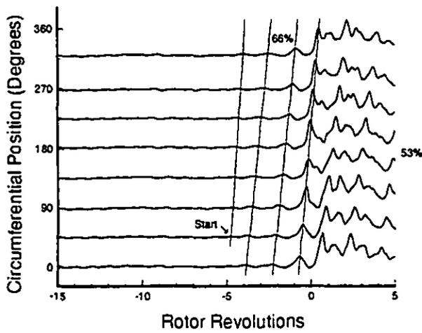
Figure 13. Stall Inception at 98.6% Speed Circ Grooves
