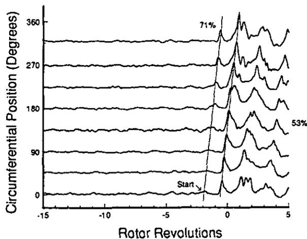
Figure 17. Stall Inception at 85% Speed Recirc Cavity
