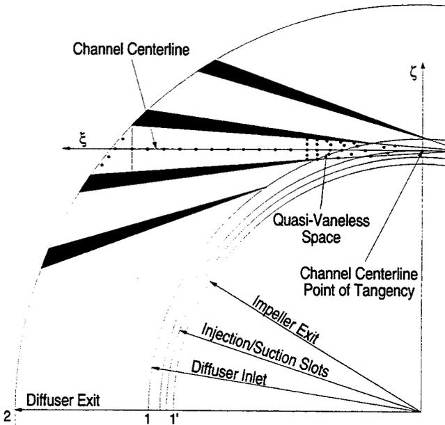
Figure 2: Straight-channel diffuser geometry and static pressure tap locations.
