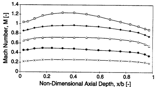
Figure 3b: Axial distributions of absolute Mach number,  $M$ , at the straight-channel diffuser inlet for different corrected impeller speeds (no injection/suction). (Same legend as Fig. 3a)
