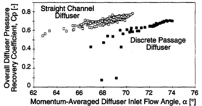
Figure 13: Comparison of mass-averaged overall diffuser pressure recovery coefficient,  $C_p$ , for straight-channel and discrete-passage diffusers.
