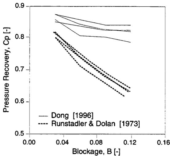
**Figure 1: Pressure recovery coefficient,  $C_p$ , as a function of inlet blockage,  $B_1$ , for single channel diffusers with different area ratios and divergence angles; comparison of the data from Dong (1996) ( $C_p$  is based on mass-averaged diffuser inlet total pressure) and Runstadler and Dolan (1973) ( $C_p$  is based on diffuser inlet centerline total pressure).**
