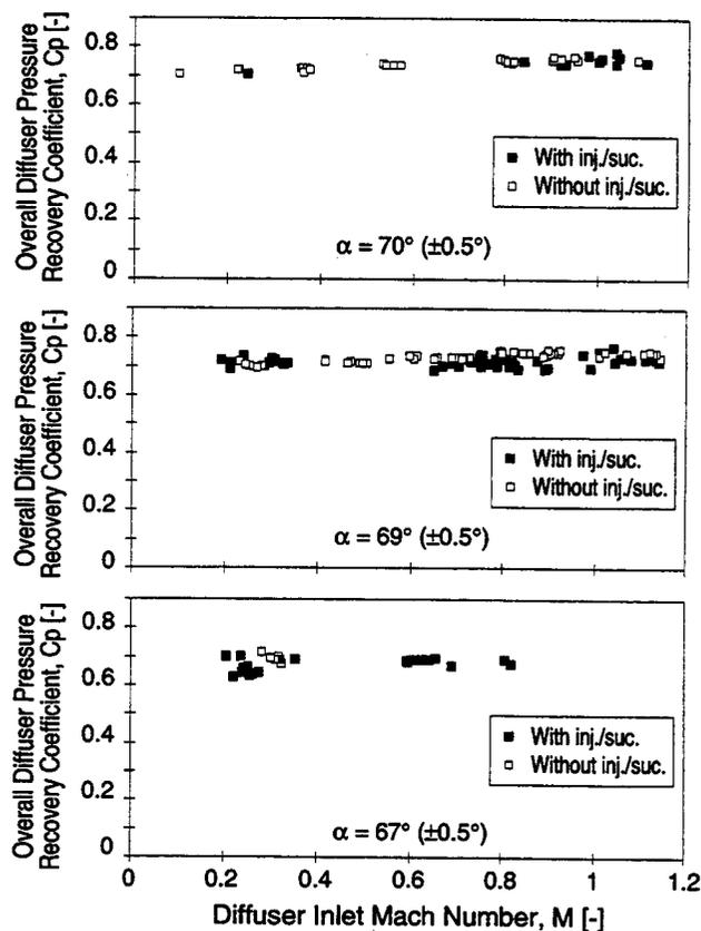
**Figure 9: Mass-averaged overall diffuser pressure recovery coefficient,  $C_p$ , versus diffuser inlet Mach number,  $M$ , represented for constant diffuser inlet flow angles.**
