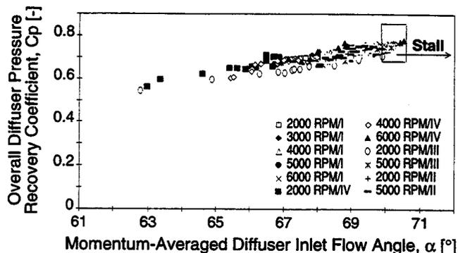
**Figure 7: Mass-averaged overall straight-channel diffuser pressure recovery coefficient,  $C_p$ , versus momentum averaged diffuser inlet flow angle,  $\alpha$ , for different corrected impeller speeds and data series (I, II, III, IV) with and without injection/suction.**
