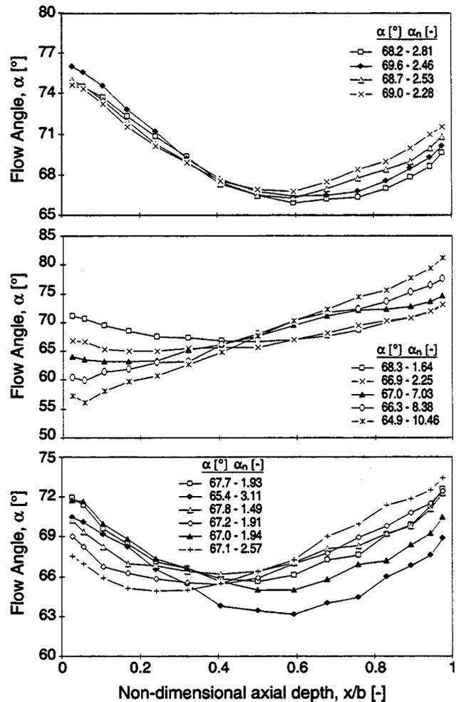
Figure 6: Examples of flow angle,  $\alpha$ , axial distribution at the straight-channel diffuser inlet (with injection/suction): a) Series II,  $N = 5000$  RPM, b) Series III,  $N = 2000$  RPM, c) Series IV,  $N = 4000$  RPM.
