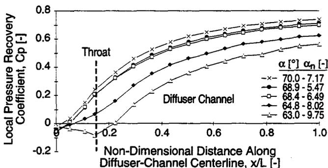
Figure 12: Static pressure distribution along the centerline of a straight-channel diffuser channel for different flow angles at a constant impeller speed  $N = 2000$  RPM (with injection/suction).
