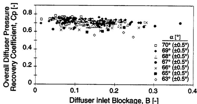
**Figure 8: Mass-averaged overall straight-channel diffuser pressure recovery coefficient,  $C_p$ , versus diffuser inlet blockage,  $B$ , with and without injection/suction.**
