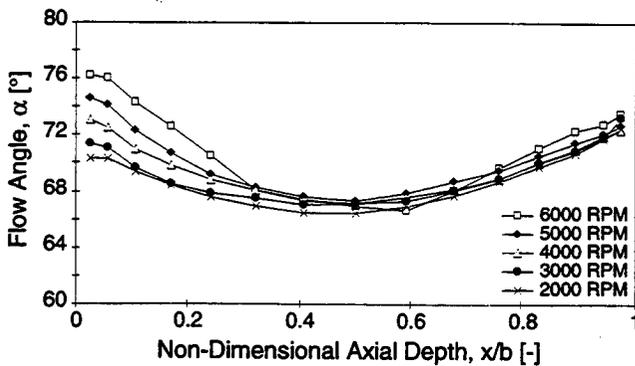
Figure 3a: Axial distributions of flow angle,  $\alpha$ , at the straight-channel diffuser inlet for different corrected impeller speeds (no injection/suction).
