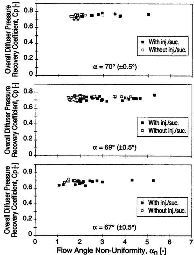
Figure 11: Mass-averaged overall diffuser pressure recovery coefficient,  $C_p$ , versus diffuser inlet flow angle non-uniformity,  $\alpha_n$ , represented for constant diffuser inlet flow angles.
