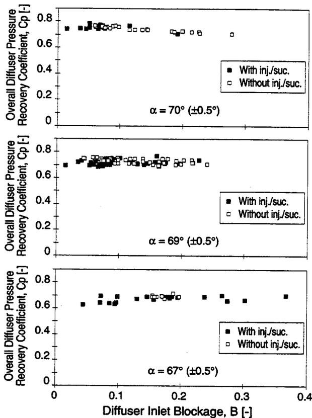
Figure 10: Mass-averaged overall diffuser pressure recovery coefficient,  $C_p$ , versus diffuser inlet Blockage,  $B$ , represented for constant diffuser inlet flow angles.
