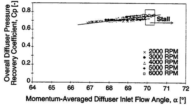
Figure 4: Mass-averaged overall straight-channel diffuser pressure recovery coefficient,  $C_p$ , versus momentum averaged diffuser inlet flow angle,  $\alpha$ , for different corrected impeller speeds (no/injection/suction).
