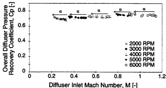
Figure 5: Mass-averaged overall straight-channel diffuser pressure recovery coefficient,  $C_p$ , versus diffuser inlet Mach number,  $M$ , for different corrected impeller speeds (no/injection/suction).
