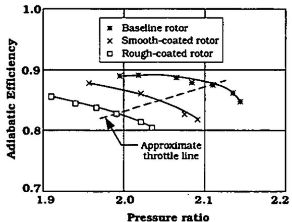
FIGURE 6. EFFICIENCY-PRESSURE RATIO CHARACTERISTICS AT DESIGN SPEED
