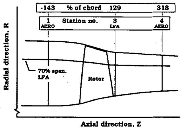
FIGURE 2. LASER ANEMOMETER AND AERODYNAMIC SURVEY STATIONS
