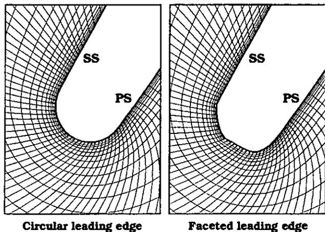
FIGURE 16. CFD GRID DETAIL AT THE LEADING EDGE
