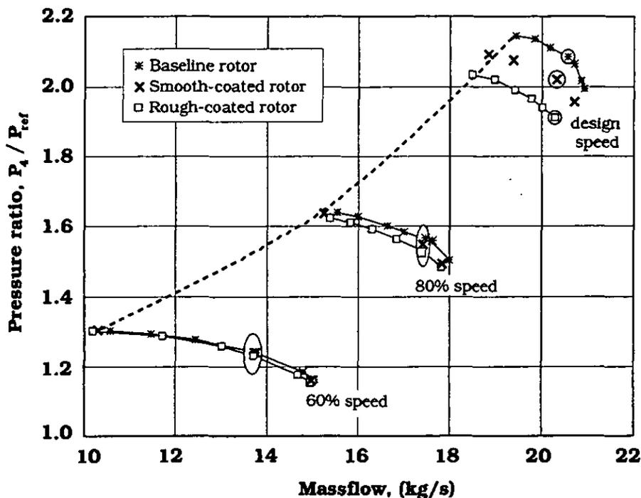
FIGURE 4. PRESSURE RISE CHARACTERISTICS FOR FULL- COVERAGE COATINGS. CIRCLED POINTS INDICATE OPERATING CONDITIONS FOR WHICH RADIAL OISTRIBUTIONS OF FLOW PROPERTIES ARE PRESENTEO
