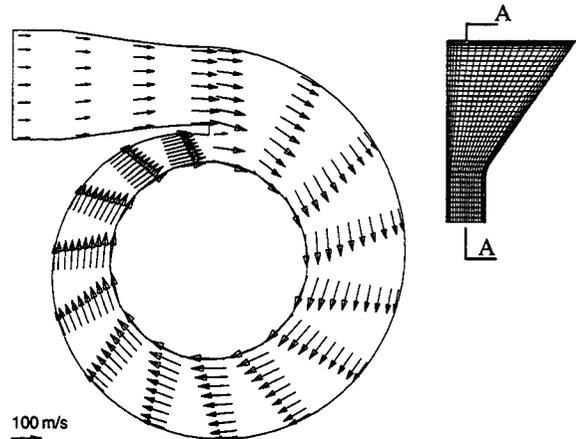
FIGURE 6a: Velocity Vector on an Azimuth Plane A-A
