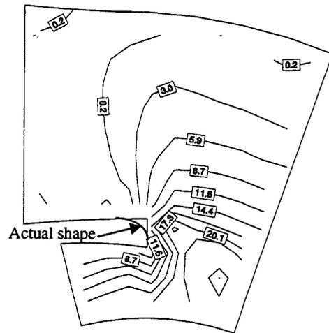
FIGURE 12: Flow Angle Distribution Around the Tongue
