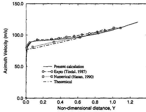
FIGURE 7b: Comparison of Azimuth Velocity at  $\theta=180$  deg
