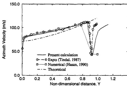
FIGURE 7a: Comparison of Azimuth Velocity at  $\theta=2.4$  deg
