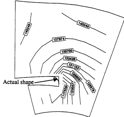
FIGURE 11: Static Pressure Distribution Around the Tongue
