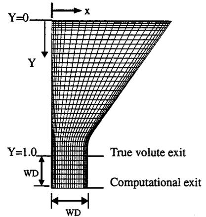
FIGURE 5b: Grid Distribution at a Cross-section ( $40 \times 24$ )
