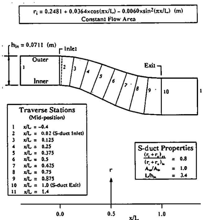
FIGURE 1 S-SHAPED DUCT GEOMETRY AND MEASUREMENT TRAVERSE PLANES
