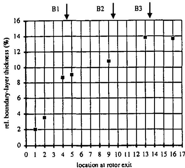
FIGURE 9: DEVELOPMENT OF CASING WALL BOUNDARY LAYER
