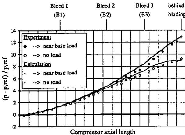
FIGURE 12: STATIC PRESSURE DEVELOPMENT AT THE CASING WALL
