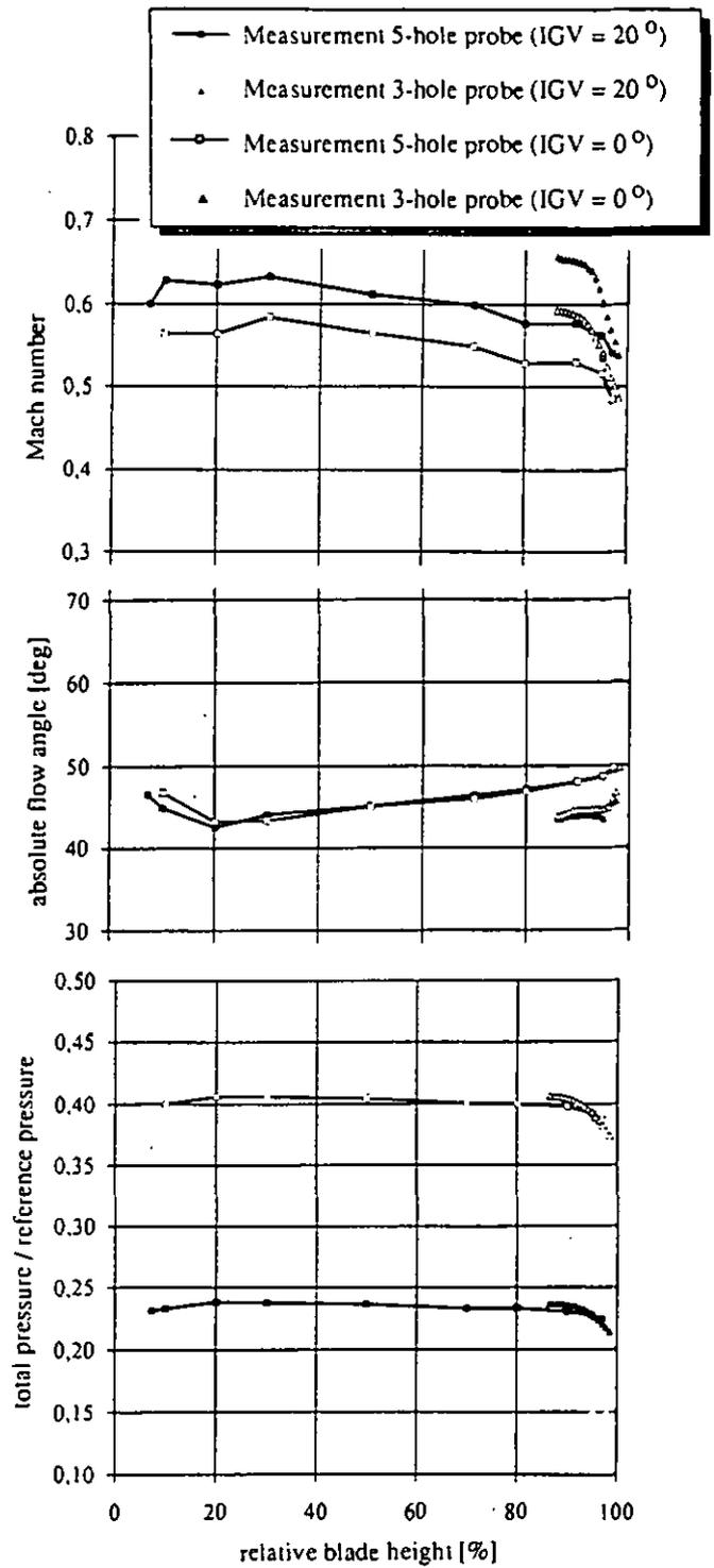
FIGURE 7: 3-HOLE AND 5-HOLE MEASUREMENTS UPSTREAM OF STATOR 9
