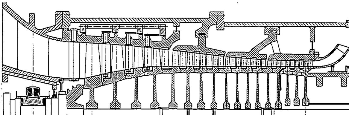
FIGURE 1: CROSS SECTION OF THE V84.3 COMPRESSOR
