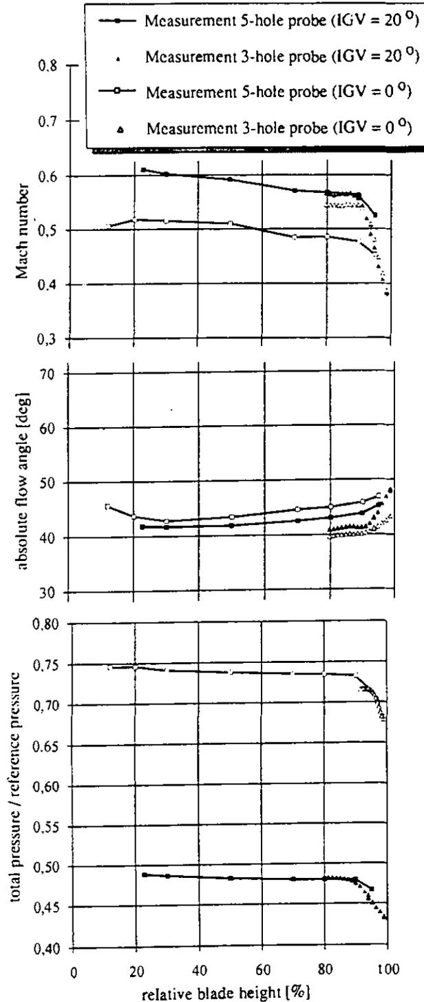
FIGURE 8: 3-HOLE AND 5-HOLE MEASUREMENTS UPSTREAM OF STATOR 16
