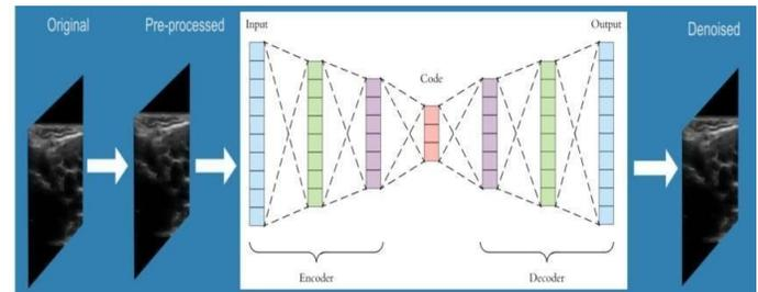
Fig. 2: Autoencoder Architecture
