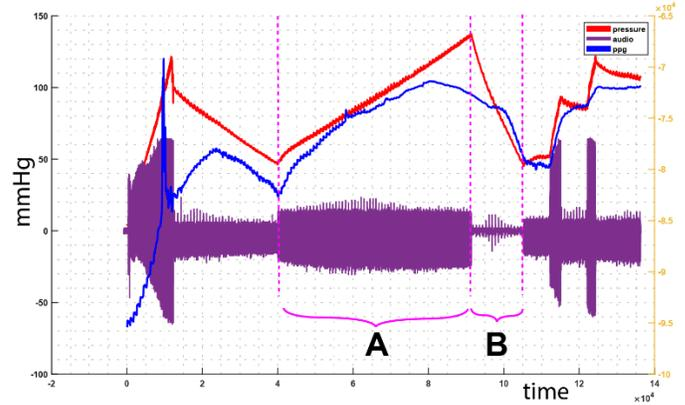
**FIGURE 3:** RAW SIGNALS PLOTTED IN REAL-TIME BY THE MATLAB PROCEDURE. SECTION 'A' ILLUSTRATES AN INFLATIONARY CURVE AND SECTION 'B' A DEFLATIONARY CURVE (MOST COMMONLY USED IN BP METERS).
