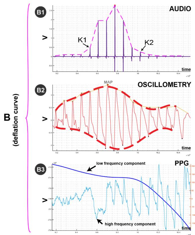
**FIGURE 5:** SECTION 'B' DESCRIBES THE BEHAVIOR OF OUR ALGORITHM IN THE DEFLATIONARY CURVE. SECTION B1 SHOWS THE DEFLATIONARY KOROTKOFF SOUNDS. B2 DISPLAYS THE OMWE WHILE DEFLATING THE CUFF AND B3 DISPLAYS THE TWO FREQUENCY COMPONENTS OF THE PPG SIGNAL.
