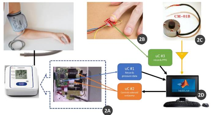
**FIGURE 2:** GENERAL DEVICE DIAGRAM. THE DEVICE HAS THREE MAIN INPUT COMPONENTS: A PRESSURE SENSOR (2A), AN OXIMETER (2B), AND A CONTACT MICROPHONE (2C). ALL THE INPUTS ARE COMBINED AND THEN ANALYZED USING MATLAB (2D).
