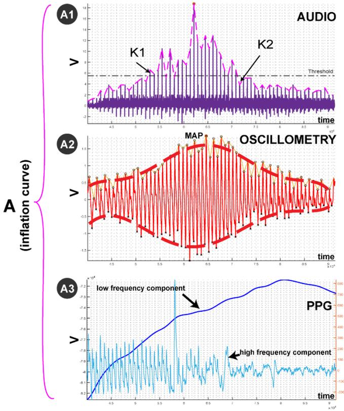
**FIGURE 4:** FIGURE 4A SHOWS THE KOROTKOFF SOUNDS, FIGURE 4A2 DEPICTS OSCILLOMETRY, AND FIGURE 4A3 SHOWS PPG SIGNALS OUT OF THE INFLATIONARY CURVE FROM SECTION 'A' IN **FIGURE 3**.
