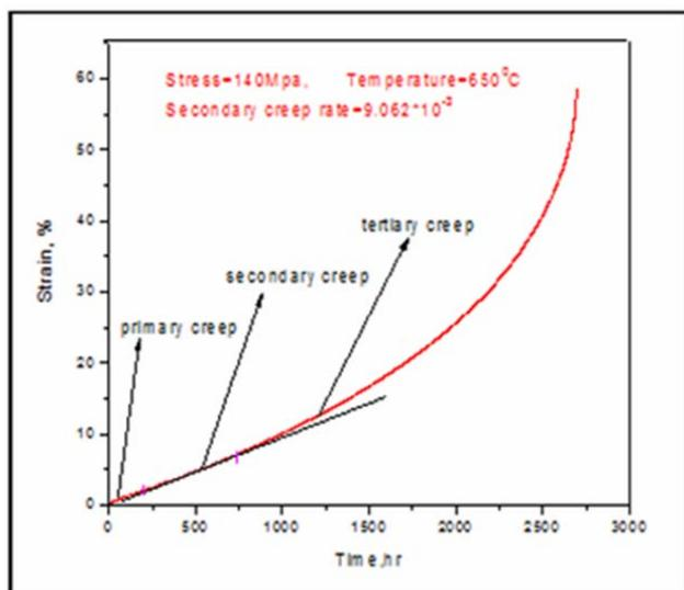
Figure 10. Creep behavior of SS 316 from literature indicates ~2% creep strain after 200 hours at 650C (1200F) at 140 MPa (20 ksi)<sup>5</sup>.
