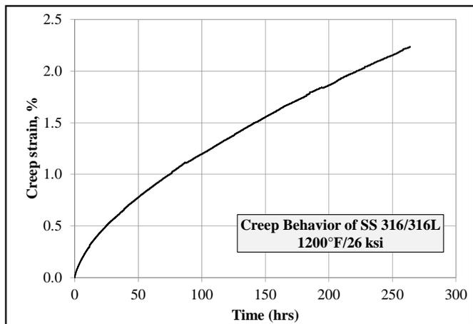
Figure 9. Creep curve of hot extruded 316/316L stainless steel at 1200F/26ksi/260hours.
