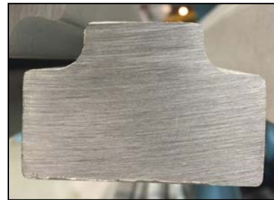
Figure 4. Extruded and straightened sections of SS316 used for valve bodies utilized for a variety of industrial applications.
