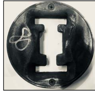
Figure 3. Modified tool steel die, manufactured in-house, used for stainless steel extrusion process.
