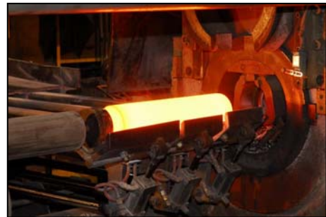
Figure 1. Forward extrusion process at PES, where the ram ‘pushes’ the hot metal through the die.
