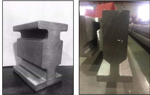
Figure 3. Modified tool steel die, manufactured in-house, used for stainless steel extrusion process.
