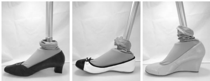
FIGURE 1: A PROSTHETIC FOOT ALIGNED FOR ONE PARTICULAR HEEL RISE (LEFT) IS INHERENTLY MISALIGNED WHEN WEARING SHOES OF OTHER HEEL RISES, AS DEMONSTRATED BY THE ANGLE OF THE RESPECTIVE PYLONS (CENTER, RIGHT).
