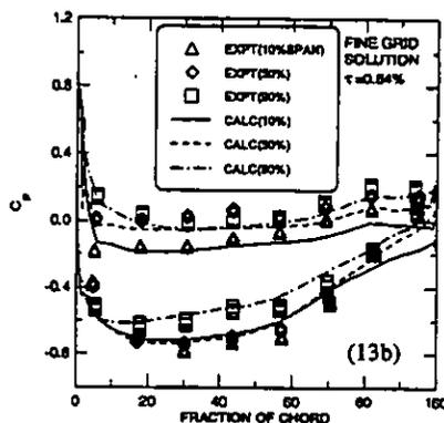
Figure 12. Blade surface pressure in the spanwise direction
