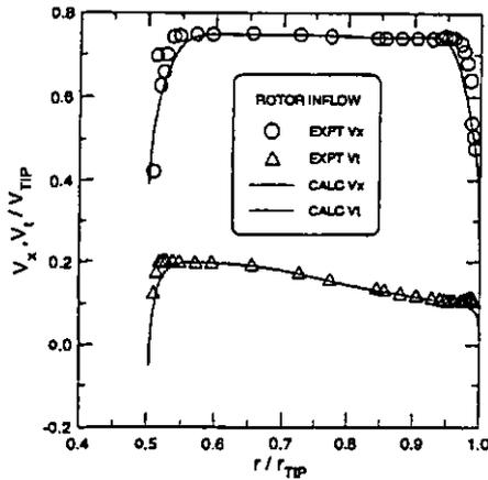
Figure 8. Inflow velocity for pump rotor
