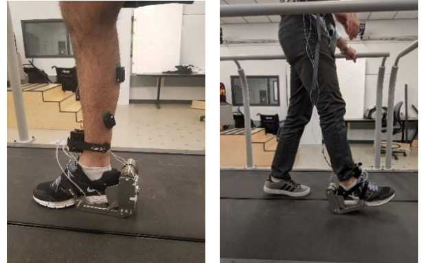
FIGURE 7: SUBJECT WALKING ON TREADMILL WITH THE ROBOTIC SHOE (LEFT) AND EMG PLACEMENT (RIGHT)
