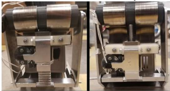
**FIGURE 3: ROBOTIC SHOE LOCKING MECHANISM**
