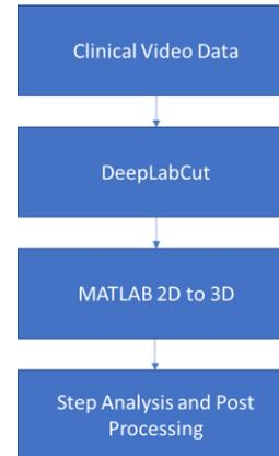
**FIGURE 1:** THIS FIGURE SHOWS THE PROCESS FLOW FOR TAKING THE RAW VIDEO TO 3D DATA AND FINALLY POST PROCESSING.
