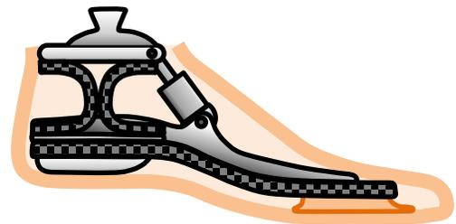
**Figure 5. Dual “C” spring model with cylinder.**
