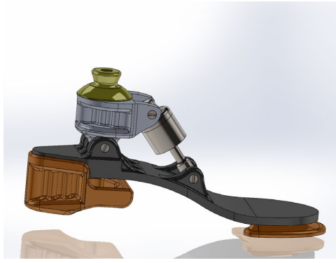
Figure 6. Single-axis implementation with cylinder.
