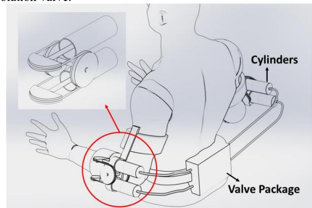
Figure 1. Body-powered wearable robot
