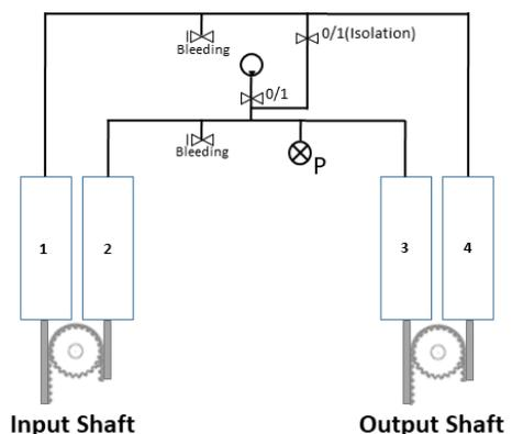
Figure 2. Antagonist transmission circuit with a 1:1 transmission ratio.
