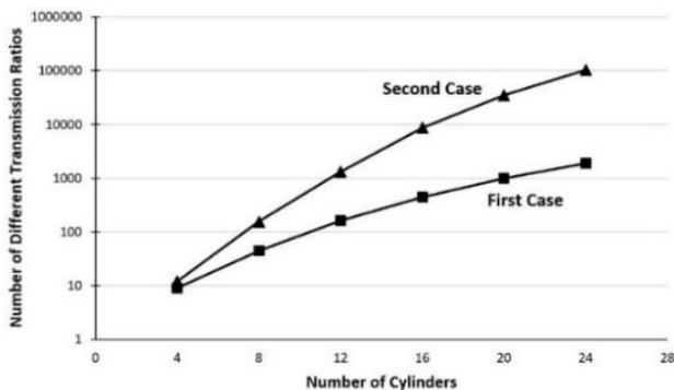
Figure 6. The number of unique transmission ratios with respect to the number of cylinders for two assumptions; first assumption: similar cylinder sets with the output pulley sizes similar to the input pulley sizes, second assumption: unique size for all cylinders and pulleys in the system.
