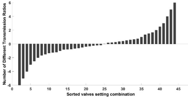
Figure 5. Transmission ratios using eight cylinders and 16 valves
