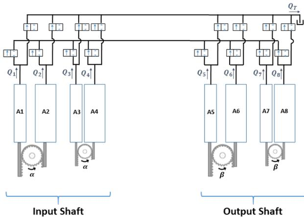
Figure 3. Variable hydraulic transmission with eight cylinders and sixteen valves
